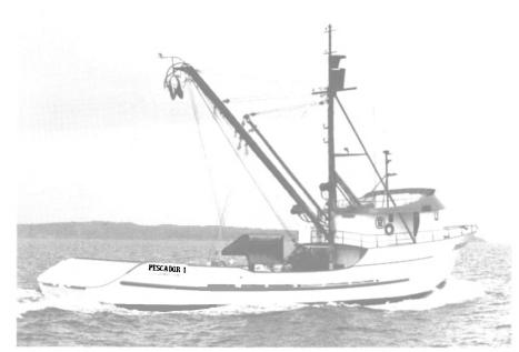
Pescador I by MARCO is powered by a Caterpillar D398TA diesel driving a Coolidge
