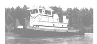
The 60-foot push boat 'Bengal Phil' was recently delivered by Bayou Black Shipyard to Hillman Marine. tage of the aluminum construction will be in the minimum maintenance time on the superstructure.
