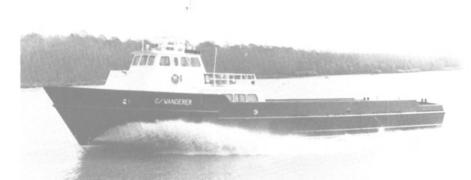
MTU-powered M/V C/Wanderer, a new crew/supply vessel designed and built by Swiftships, Inc. of Morgan City, La.
