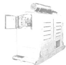
30KW Delco generator—80% P.F. GMC 3-71 diesel has 24 volt electric starter, with oil, amps & temp gauges, alternator and muffler. Generator equipped with main circuit breaker, voltage regulator, voltmeter, ammeter, frequency meter. 220/440/3/60—1200 RPM. Dry weight 4950 lbs. 100" long x 34" wide x 78" high.
