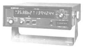
Loran C Coordinate Converter Model TC-28A adds total navigation functions to most Simrad Loran C Receivers. Converts TD's to Lat/Long, memorizes up to ten waypoints and calls up course and distance to any of them. Computes and displays on command time to destination and cross-track error. Installs directly on TL-838 or separately with other Simpod and the Molecular Management of the contraction of the con with other Simrad models. Makes them all navigators.
