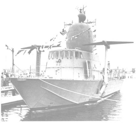
Grumman hydrofoil patrol craft built at Lantana Boatyard, Inc. in Florida was launched recently. An improved version of Grumman-designed Flagstaff (PGH-1), vessel is powered by 5,400-hp Allison gas turbine engine, can attain 50-knot speed.
