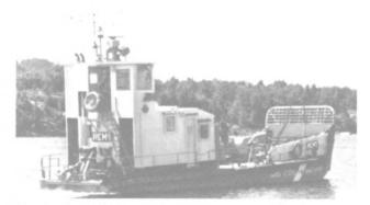
2.Landing Craft, M.V. Remy, built 1943. Powered by two G.M. Diesels, 175 H.P., 52' long, 14' wide, 4'6" draft, c/w McDougall Water Pump with Briggs and Stratton Engine, 4 cycle, 1 cylinder, 3 H.P. Location: Parry Sound, Ontario
