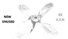
Starboard -7' diameter - pitch constant 4.699: Bore tapers from 6½" to  $4^{53}/_{4}$ ".  $141/_{2}$ " taper equal to 1"/foot on diameter. U.S. Navy reconditioned. Average weight 1760 lbs.
