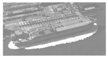
BELCHER 102-BIG AND VERSATILE. The belcher 102-BIG AND VERSATILE. The biggest barge ever built in this country for the transportation of oil and probably the largest ever constructed anywhere for the movement of petroleum products. Double skinned with dimensions of 640 feet long by 105 feet wide and 48 feet deep, she has a capacity of 55,000 DWT or 412,000 barrels.
