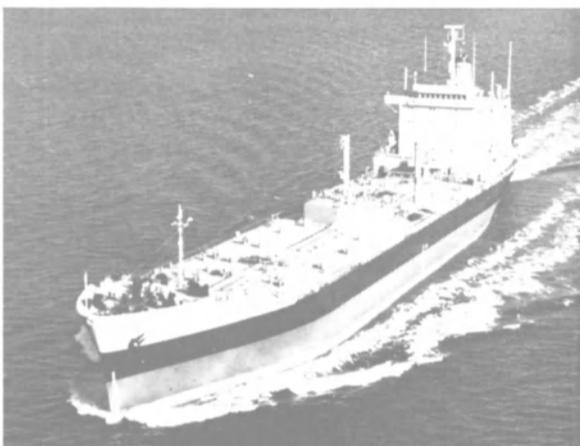
Similar to the two tankers for which Transamerica Delaval will provide main propulsion engines is this Falcon I-MSV vessel which entered service in 1975. Twin Delaval diesels power the original ships—a fleet of five. The two new tankers will be equipped with the same engines: Delaval "Enterprise" RV-16, medium-speed diesels. Each 16-cylinder unit is rated at 7,360 bhp.
