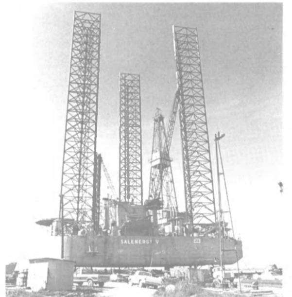
Downtime was cut by half when dockside repairs on the jackup drilling rig Salenergy V (shown above) were completed by Industrial Marine Services in Cameron, La. The interval between the rig's arrival at Industrial Marine and the day the work was completed on schedule was approximately half the repair time that would have been required if the rig had been repaired in the Gulf. The rig will begin initial drilling operations for ARCO off Morgan City, La., in the Gulf of Mexico.
