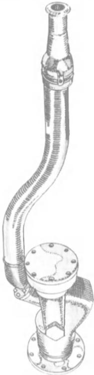
and featuring simple design, the MP provides the very high reliability required for within-tank mounting. This single nozzle tank cleaning machine weighs 178 lbs and can be fixed-in-place in any location, at any angle, and is specifically designed to allow installation on tank bottoms under the cargo. *The MP advantage:* cleans large areas which cannot be reached by conventional deck-mounted equipment and provides unbeatable Butterworth Systems performance.
