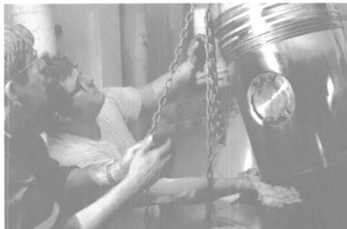
Close inspection of the piston skirts found them clean and smooth, with no scoring.
