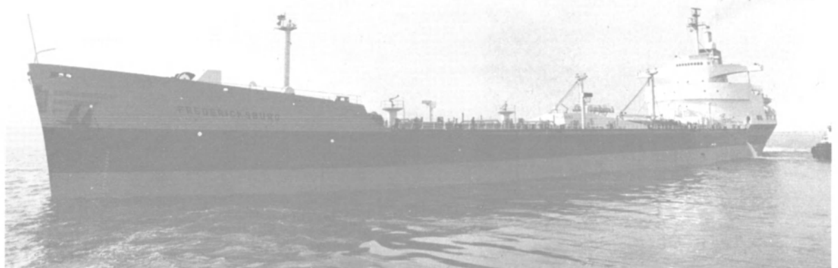
Jumboized tanker Fredericksburg now has superstructure full aft, and is 24 feet longer, 19 feet wider, and capable of carrying some 110,000 more barrels of oil.
