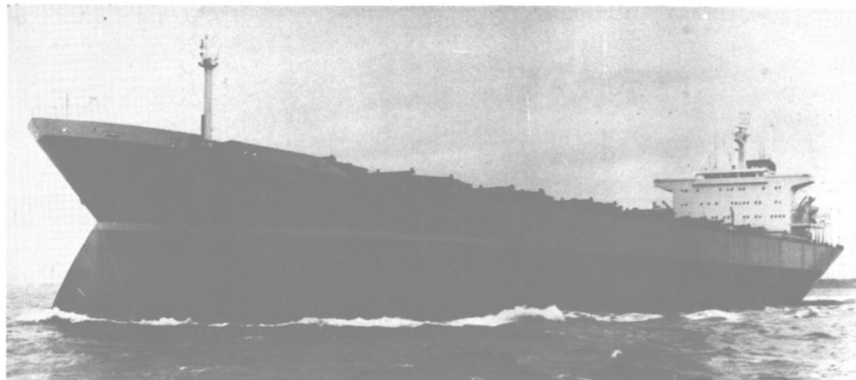
The 64,000-dwt Danelock, first bulk carrier of Burmeister & Wain's fuel-saving Panamax type, was delivered recently by the Copenhagen shipyard. Her power plant is a slow-speed B&W 5L80GFC diesel producing 12,600 bhp at 90 rpm.
