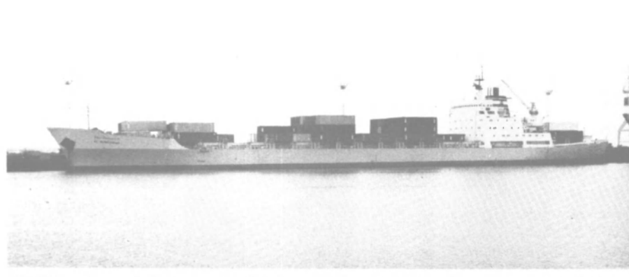
AFTER — Converted ships are 592.92 feet LOA, 15,000 dwt, capacity of 800 TEUs.
