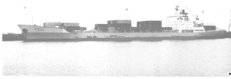
AFTER — Converted ships are 592.92 feet LOA, 15,000 dwt, capacity of 800 TEUs.
