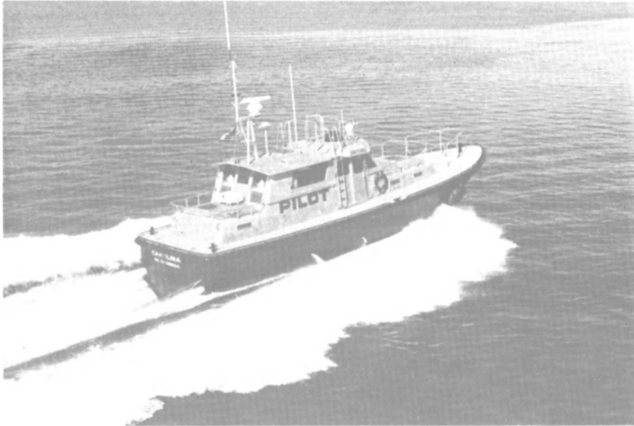
Aluminum pilot boat Carolina , designed by C. Raymond Hunt Associates and built by Gladding-Hearn Shipbuilding, was delivered recently to the Charleston (S.C.) Branch Pilots Association. High-speed vessel is powered by twin Detroit Diesel 8V92 turbocharged engines.
