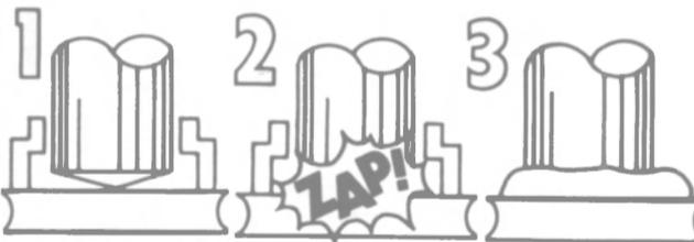
1. The fastener is placed against the work.
