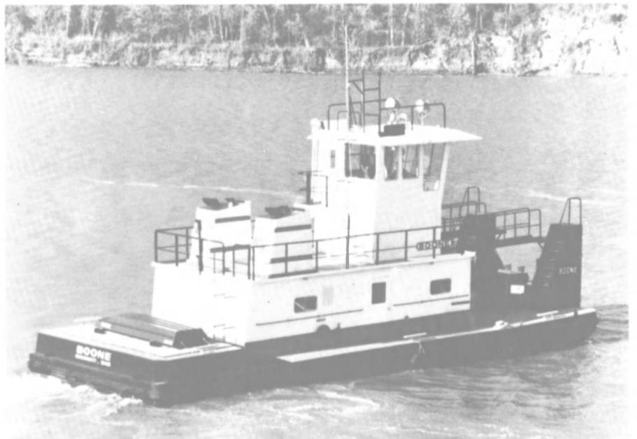
The M/V Boone, shown above, is powered by twin Caterpillar 3412 marine engines. The vessel, built by Dravo SteelShip, was recently delivered to Cincinnati Gas and Electric for use at their coal and lime facility on the Ohio River.
