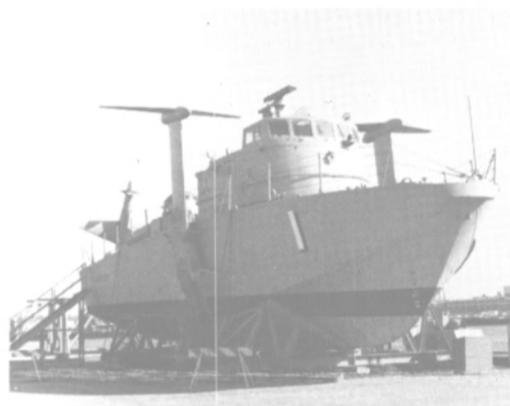
LENGTH: 74.4' OVERALL; BEAM: 21.4' EXTREME; DRAFT: MAX 4.5' SITTING 13.5' FOILS DOWN; DISPLACEMENT 56.8 FULL LOAD; CONDITION: VESSEL IS INCOMPLETE. PARTS AND ITEMS MISSING. THE PARAMETERS DESCRIBE THIS VESSEL WHEN IT WAS NEW, NOT AS IT IS NOW. VESSEL IS SOLD "AS IS, WHERE IS." WE URGE BIDDERS TO INSPECT.
