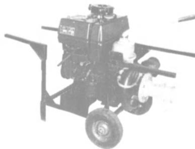
ENGINE: Mfg. by V.M.—air-cooled model HR192A—13.5 HP—3000 RPM—rope start (crank optional). PUMP: Hale—cast iron—3"—N.P.T.—hand priming—weight 410 lbs. Carrier mounted with 2 pneumatic tires for easy handling or 2-man hand carry. Ideal for oil barge, tankers, dockside, etc use.
