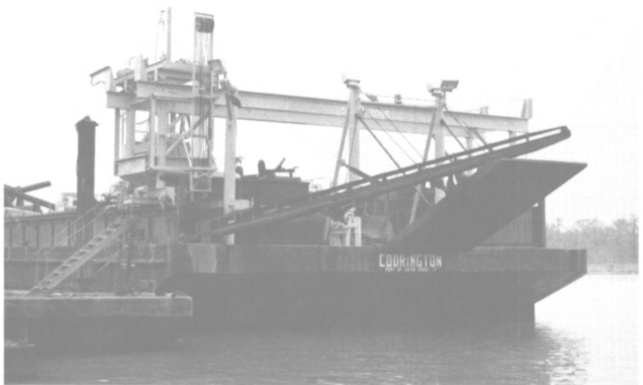
Red Jacket Mines' giant, self-unloading sand barge Codrington, built at Wall Shipyard, shown in New Orleans shortly before it left for the Caribbean.
