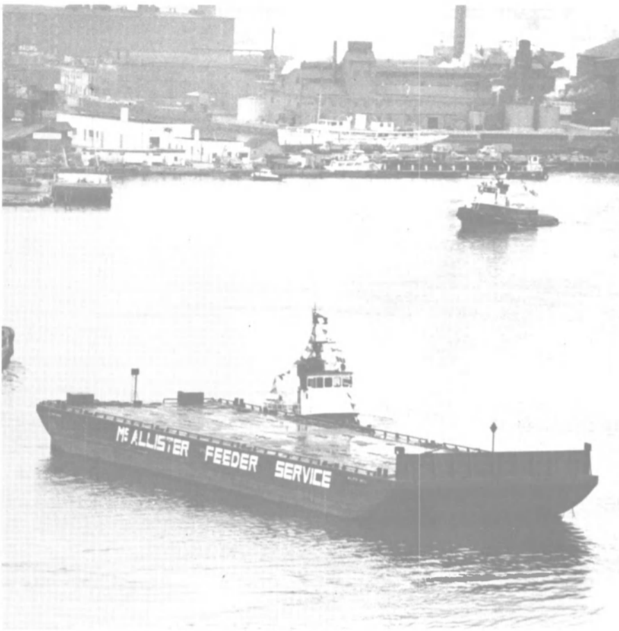
Container Feeder Service barge McAllister Shuttle can be loaded with 192 twenty-foot units. New feeder service will link Baltimore with Philadelphia and Norfolk.
