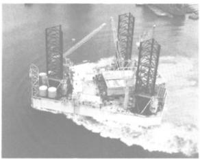
DRILL RIG LAUNCHED — Marathon Le-Tourneau Company's Gulf Marine Division recently launched this Marathon Class 82-SD-C cantilever jackup drilling rig at its Brownsville, Texas, yard, where it is currently being outfitted for its owner, Keyes Offshore, Inc., Houston. The new Marathon-built rig is designed for 20,000-foot drilling depths in water depths up to 250 feet. The Keyes rig is scheduled to be christened on May 30 as the "Keyes 250."
