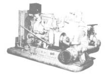
Driven by GM 3-71 diesel engine. PUMP: 1000 GPM @ 150 PSI/1500 GPM @ 100 PSI — 1750/2000 RPM. Maximum 175 PSI. Self-contained fuel tank in base. Automatic self-priming optional.
