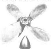
Starboard – 7' diameter – pitch constant 4.699: Bore tapers from  $6\frac{1}{6}$ " to  $4\frac{3}{6}$ 4".  $14\frac{1}{2}$ " taper equal to 1"/foot on diameter. U.S. Navy reconditioned. Average weight 1760 lbs.
