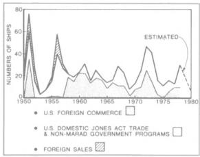
Figure 1 — Merchant vessels of 1,000 gt and over contracted for with private U.S. shipyards, net of cancellations, showing distribution between three markets.
