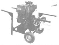
ENGINE: Mfg by V.M.-model HR192A-13.5 HP-3000 RPM -- rope start (crank optional). PUMP: Hale -- cast iron-3"-N.P.T.-hand priming-weight 410 lbs. Carrier mounted with 2 pneumatic tires for easy handling or 2-man hand carry. Ideal for oil barge, tankers, dock-
