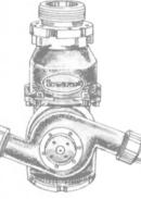
Fixed-in-place, the K machine is ideal for cleaning smaller tanks or small hard-to-clean areas in large tanks. Its twin nozzles rotate while the entire unit revolves, thereby producing Butterworth Systems' "ball of twine" pattern which ensures that every inch of surface is completely covered
