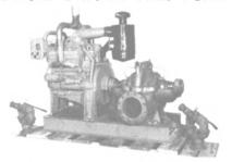
3510 GPM @ 350' HEAD or 161.7 PSI Pump: 10" x 8" horiz. split case. Diesel: GM 6V-71 or 6-71 in-line, radiator or heat exchanger cooled.
