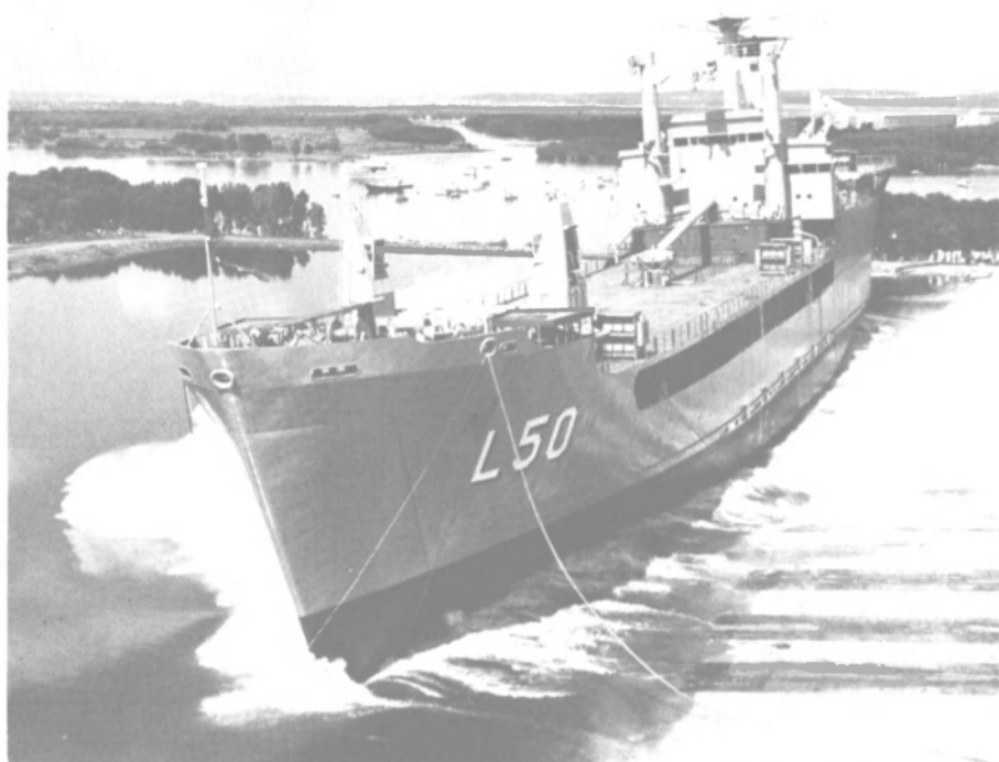
Amphibious heavy-lift ship HMAS Tobruk was side-launched into a specially constructed basin at Carrington Slipways in Tomago. Commissioning of the Royal Australian Navy ship is expected in October of this year.
