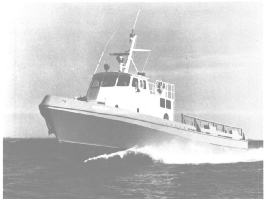
Crewboat Richard Hill is one of two delivered recently by Halter Marine's Chalmette, La., yard to P.T. Bailey, Inc. of Morgan City, La. Each boat has a capacity for up to 55 passengers, and a range of 500 miles.
