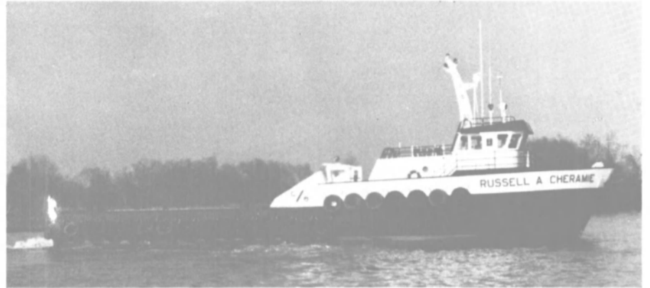
Versatile supply/utility boat Russell A. Cheramie, built by Halter for C & E Boat Rental, can also serve as survey vessel or diving tender.
