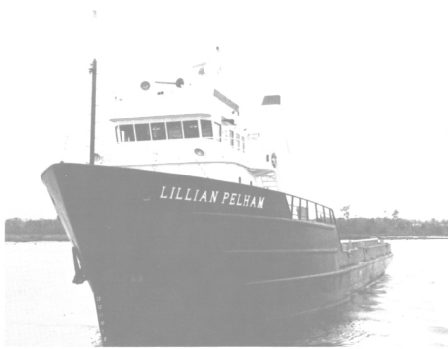
Powered by twin GM16V-149TI main engines, the 180-foot supply vessel Lillian Pelham was built by Halter Marine for Pelham Marine.
