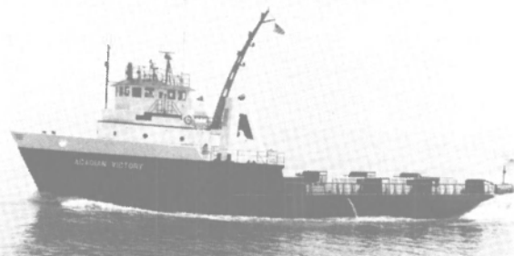
The Acadian Victory shown above is one of Acadian Marine Services' 176-foot, 3,100-hp "Freedom" class offshore supply vessels.
