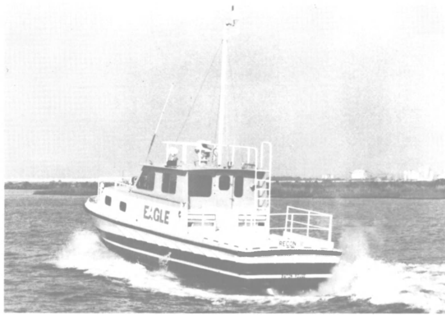
The Halter-built 14-knot survey boat Recon III is powered by two GM6-V71N engines driving Mariner 120H steerable Z-drive propulsion units.
