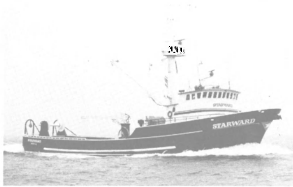
The 198-ton, 12-knot, combination boat Starward is 122 feet in overall length, with a beam of 31 feet 4 inches and a 14-foot 6-inch draft.
