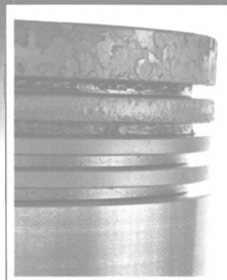
Ring groove fill normal. Number 3 and 4 lands clean.
