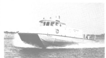
The Bell-Halter built surface-effect ship Rodolf, shown demonstrating her high speed and minimal wake, is powered by two Detroit 8V-92N engines. Her lift fan is driven by a Detroit Diesel 4-53N.
