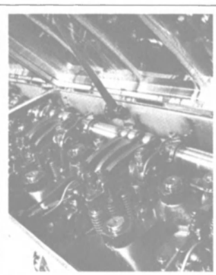
Valve deck illustrates cleanliness typical of both engines.
