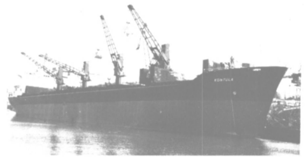
The 179-meter by 25.7-meter by 10.5-meter (about 587-foot by 84-foot by 34-foot) bulk carrier M/S Kontula is powered by a Wartsila-Sulzer 6RND76, 12,850-hp engine. Auxiliary power is provided by three Wartsila Vasa 6R22B, 1,090-hp engines.
