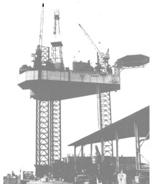
Shown here at Marathon's Singapore yard, the Pohai VIII is equipped with 360 feet of leg. The unit is capable of drilling in 250 feet of water to a drilling depth of 20,000 feet.
