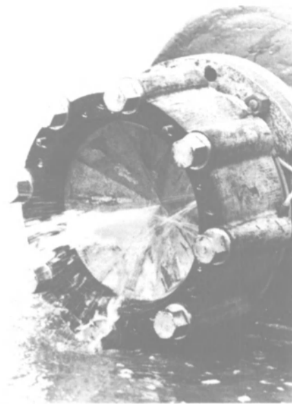
The Gall Thomson hose safety breakaway coupling is designed to avert hose breakage and reduce risk of pollution.
