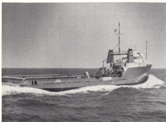
The new Brazilian-flag Ogum is powered by two EMD diesels developing 1,500 horsepower each at 900 rpm.
