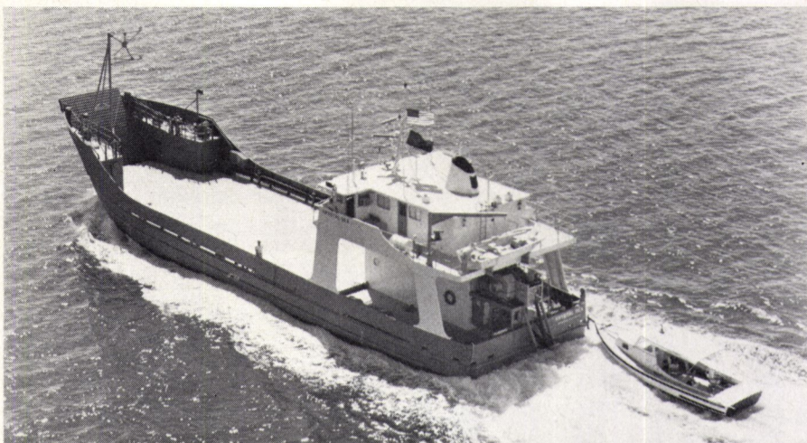
The new Arndt Brothers landing craft is powered by a pair of 365-horsepower Caterpillar 3405 diesel engines with a cruising speed of 10 knots.
