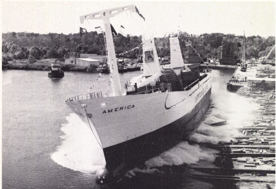
The 2,000-dwt America, shown in her side launching at Equitable Shipyards in Madisonville, La., will join a new fleet of American-flag ships serving the Caribbean and South American trades.
