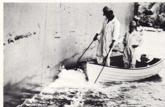
Haircut Scrubber horizontally operated from a dinghy.
