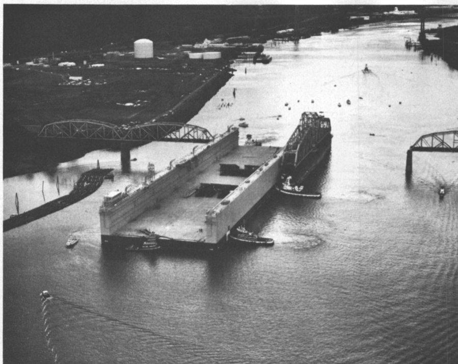
The Port of Portland's new floating drydock—the world's third largest—is eased by powerful tugboats of Willamette Tug and Barge Company through the open span of the Burlington Northern Railroad Bridge across the Willamette River in downtown Portland, Ore. The 902-foot-long structure, with a width of 229 feet 10-3/8 inches, transited the 231.6-foot-wide bridge opening with hardly a hitch, under the direction of four Columbia River Pilots—Captains Bill Ross , command pilot, Henry Childs , Don Sanford and C.D. Modrow . A nudge here, a push and pull there, a frequent "Easy does it" over the tugboats' intercoms, and in less than an hour the drydock cleared the last dolphin and continued on upriver. The floating drydock, towed from Japan by its builder, IHI Industries, and moved from Astoria more than 100 miles up the Columbia and Willamette Rivers by Willamette Tug and Barge, already is booked by the Port for repair work through the next 12 months.
