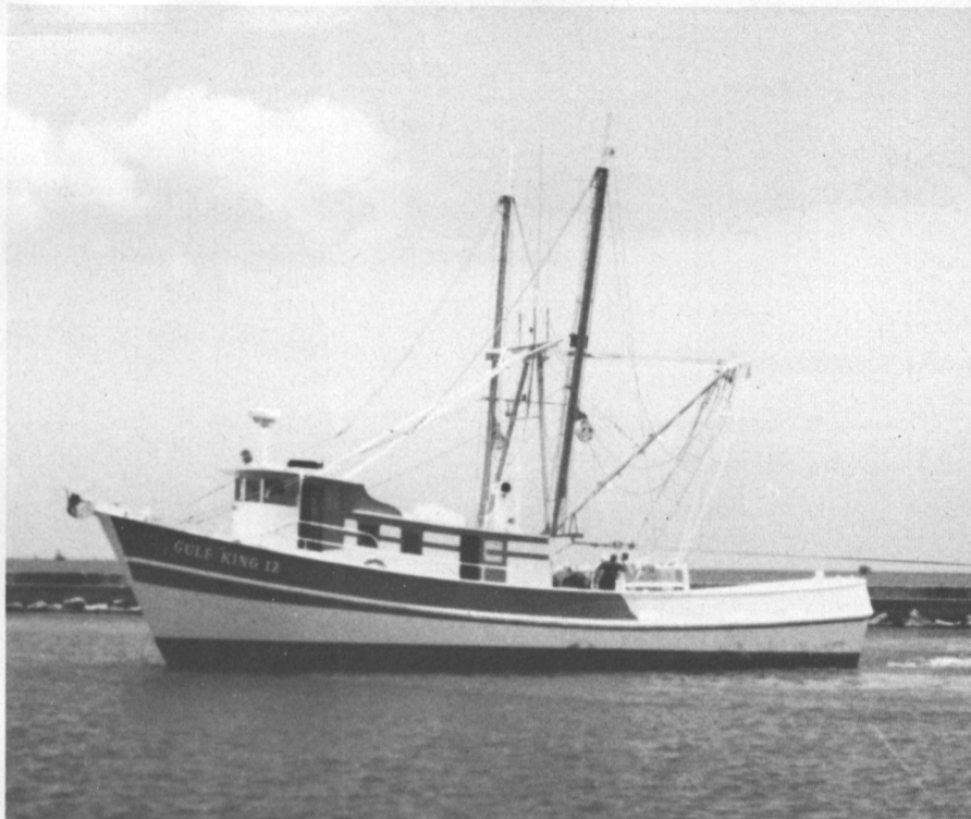
The Gulf King 12 is powered by a Kelvin Model TASC8 marine diesel engine rated at 415 shp. Her fish hold can handle 2,600 cubic feet of shrimp.
