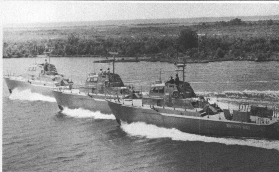
HALTER VESSELS TO THAILAND — The three all-aluminum boats shown above were delivered recently by Halter Marine, Inc., New Orleans, La., to the U.S. Government for the use of the Government of Thailand in its customs operations. They are 65 feet long, with a 17-foot beam, and 8-foot 3-inch depth. Each is powered by two Detroit Diesel 1271TI diesel engines.
