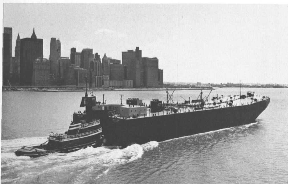
Tug Marjorie B. McAllister in notch of 18,000 ton/125,000 barrel barge. Pilot house elevated to 45' height of eye.
