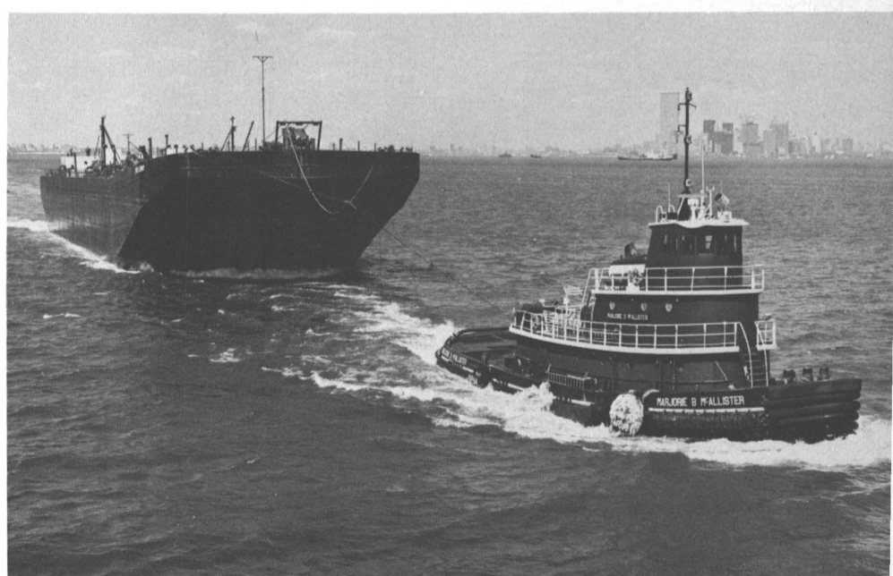
Tug Marjorie B. McAllister with barge on hawser, pilot house lowered to a conventional 28' height of eye.
