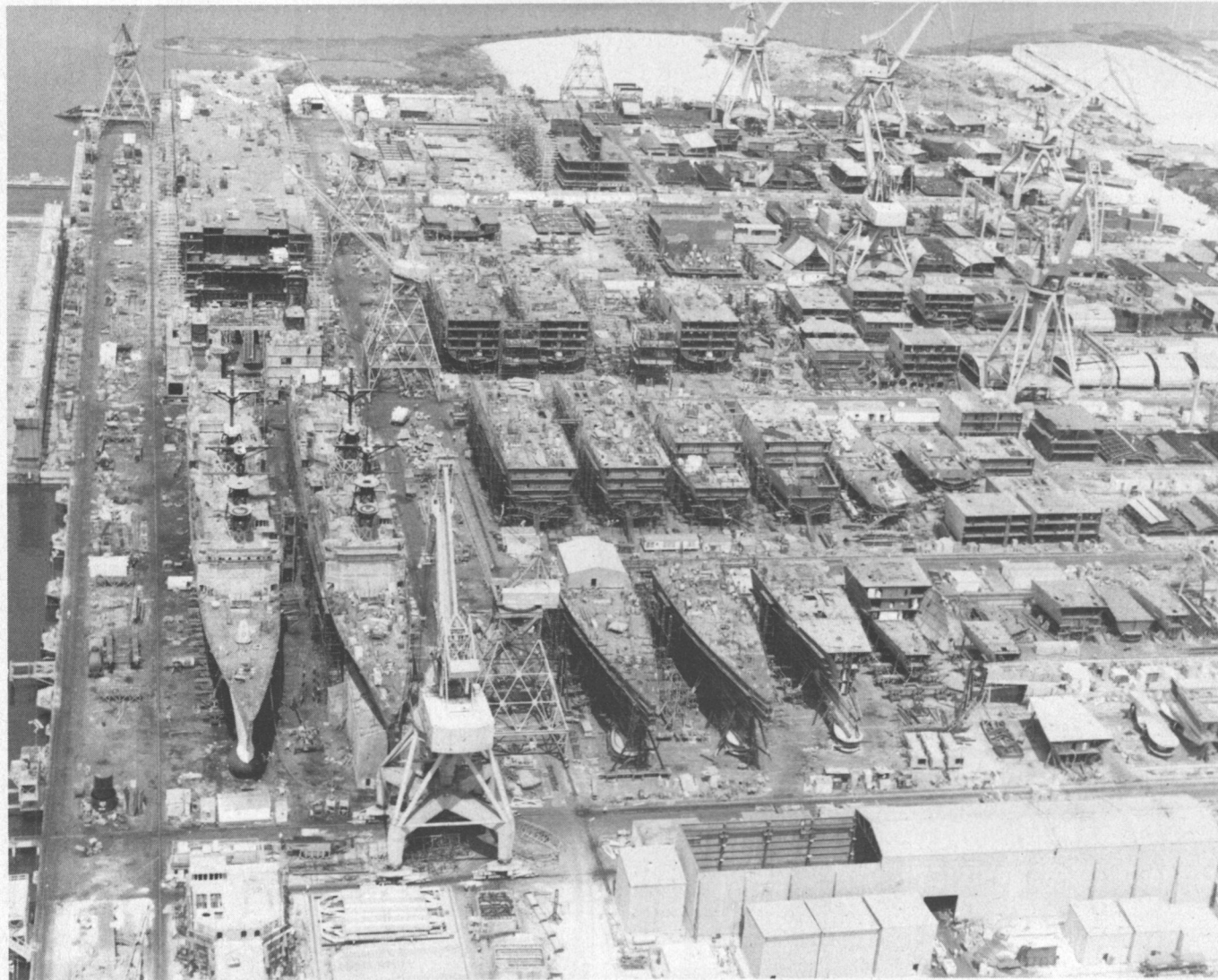
SHIP ASSEMBLY LINE —The new DDG-47 will be built at Ingalls Shipbuilding, where modular construction is currently being applied in the production of DD-963 Class destroyers and LHA-1 Class amphibious assault ships for the U.S. Navy. At least 10 combat ships are visible in this recent photograph showing the subassembly, modular assembly and ship assembly area of the Ingalls West Bank facility in Pascagoula, Miss.
