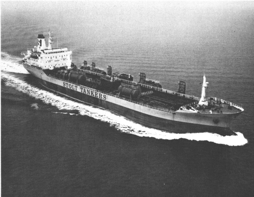
M/T Stolt Avance, sister ship of M/T Stolt Avenir. The vessel is 22,800 dwt, 560 feet loa, 32 feet 11 inches in draft, has 39 coated and stainless-steel cargo tanks, including four deck tanks, double bottom throughout, and individual hydraulically powered stainless-steel deep-well pumps and stainless-steel pipelines. These ships are certificated to carry IMCO-type I, II, and III products, and meet the highest standards of cargo, crew and environmental safety and protection.
