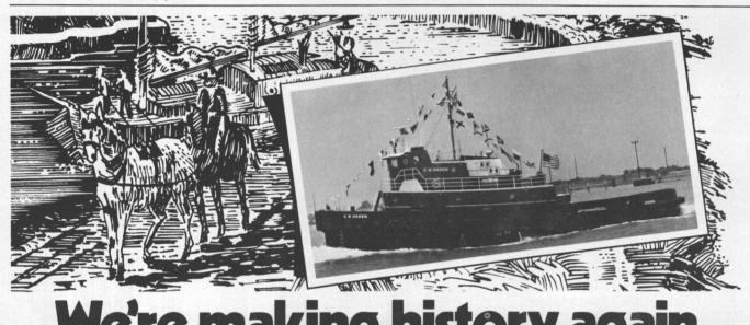
Bay-Houston announces the **C.R. Haden**, a brand new 3,200 horsepower tug with power to spare for towing, maneuvering and docking the largest vessels using Texas Gulf ports. Twin screws with Kort nozzles assure quick response to tow conditions in open harbors, narrow channels or turning basins. We've come a long way since 1880 when Captain W.D. Haden's towpath operation along upper Gal-
