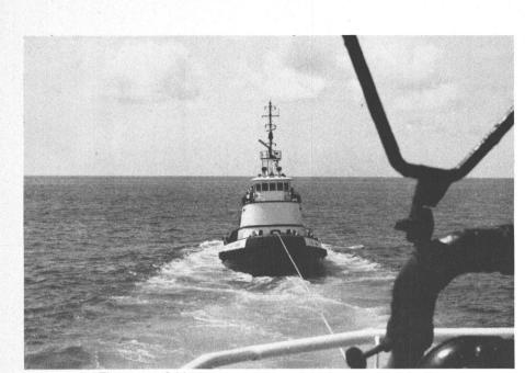
The new 6,000-hp tug Jabbar is shown utilizing the newly designed bow winches for tractor towing.
