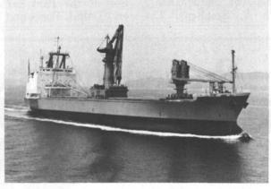
The derrick on the Malacca Maru can rotate 360 degrees while handling cargo.
