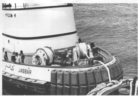
One of the most important features of the new Jabbar are the newly designed automatic line-handling winches as shown on the foredeck of the tug.
