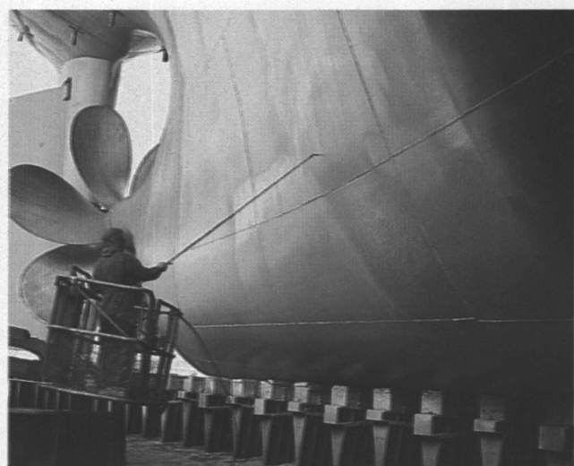
MAUI: dark area—Cathodic Protection Dielectric shield; green—first coat of SPC; blue—second coat of SPC.
