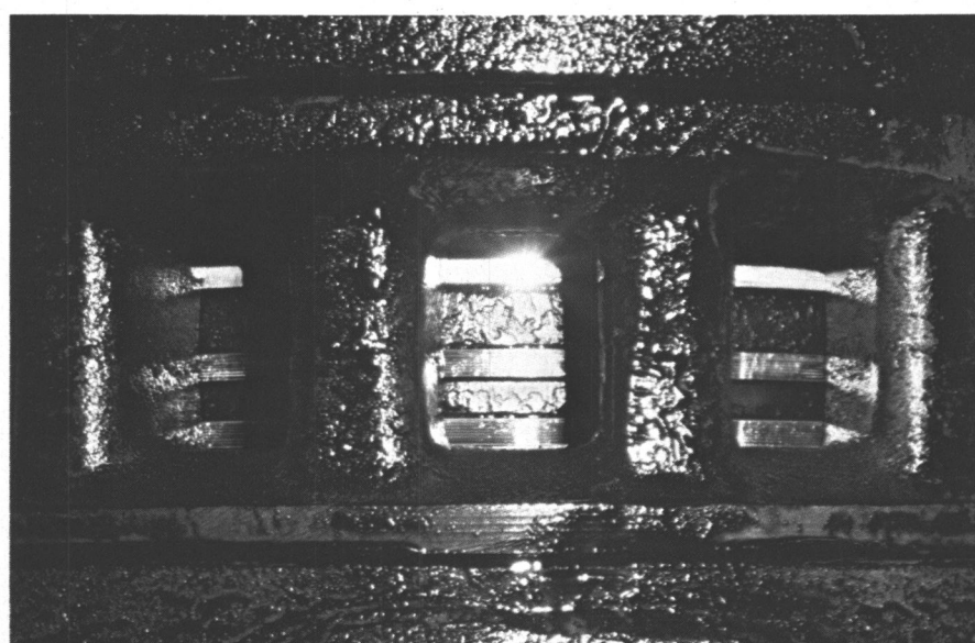
Ports are virtually 100 percent open for this cylinder after 5,564 hours on CAPRINUS R Oil 40. Average top ring side clearance .0096 inches. No chipping or scuffing of rings. CAPRINUS R Oil 40 fights deposit buildup and wear, helps lengthen the service life of critical engine parts.
