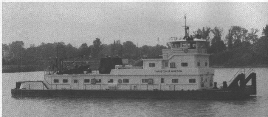
Powered by Alco diesels and designed and built by Jeffboat, the Thruston B. Morton has been constructed for use on the Illinois River, with special features which allow optimum performance year-round.
