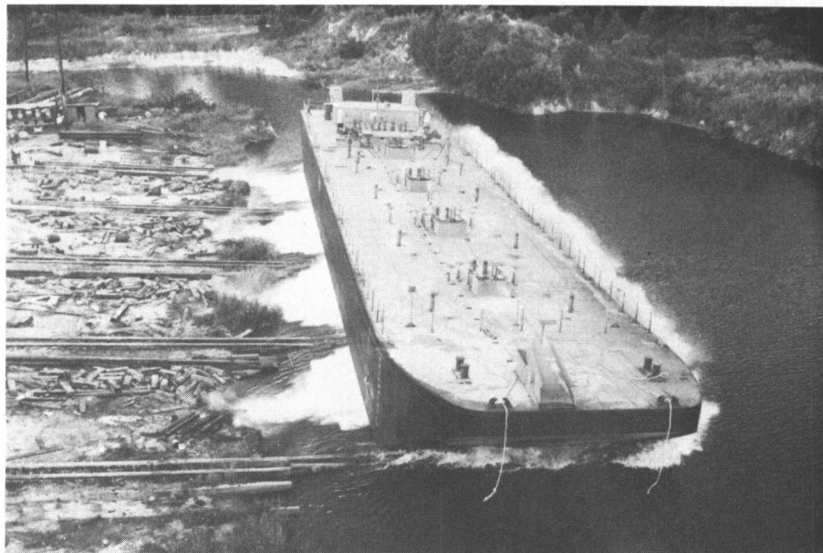
FIRST OF TWO FOR REINAUER — Equitable Shipyards, Inc., New Orleans, La.-based shipbuilder, has launched the first in a series of two oil barges for Reinauer Transportation Company, Inc., Newark, N.J. The 227-foot by 43-foot by 15-foot barges will handle Grade A and lower product. The barges are built to ABS ocean service rules and for manned service. Equitable is a wholly owned subsidiary of Trinity Industries, Inc. of Dallas, Texas, a manufacturer of industrial marine and structural metal products.
