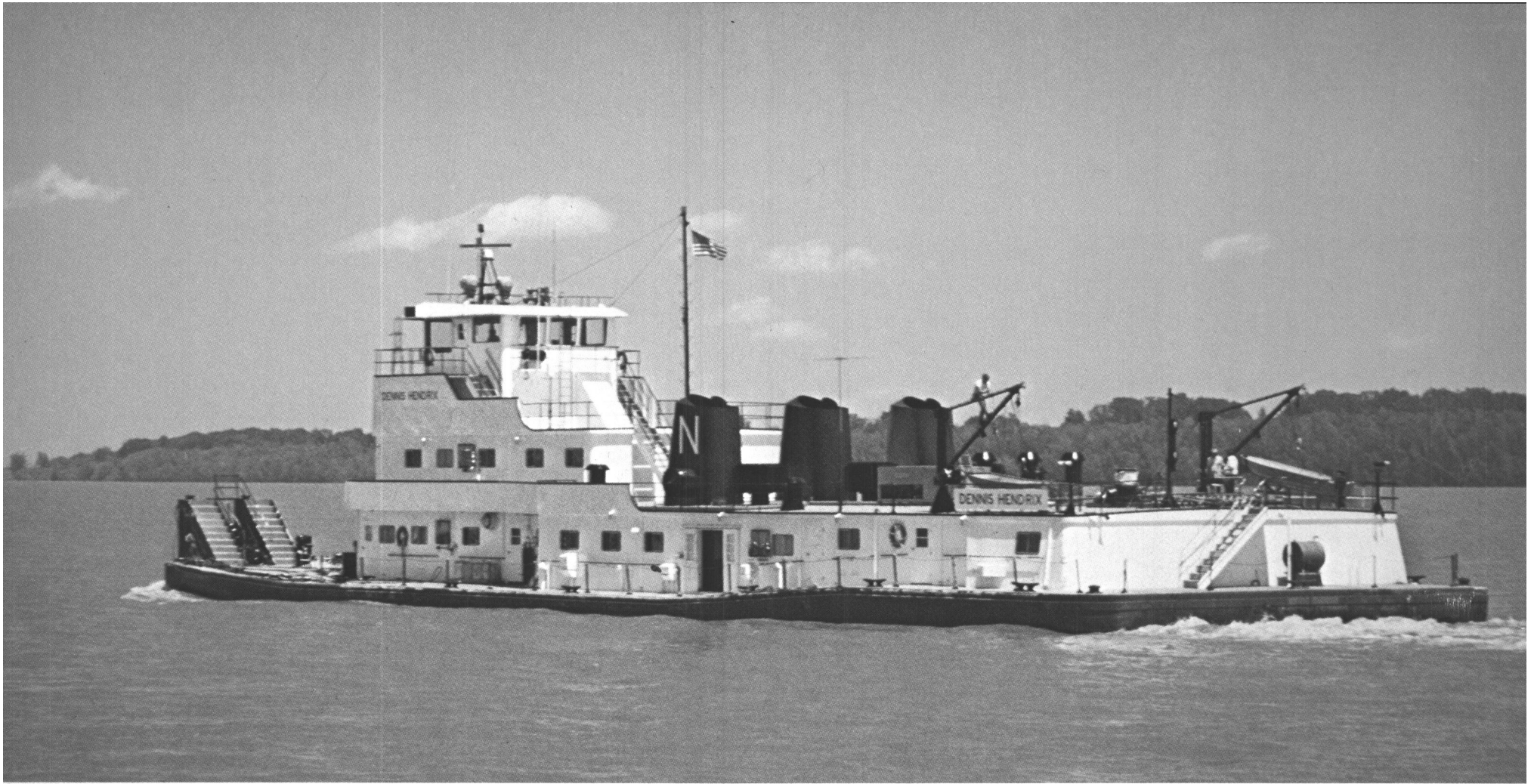
M/V Dennis Hendrix is 180 ft. long, has a 52-ft. beam and a 9-ft. draft. High-alkalinity CAPRINUS R Oil 40 is helping each of her three EMD16-645 E5's dependably deliver 2,800 hp at 900 rpm.
