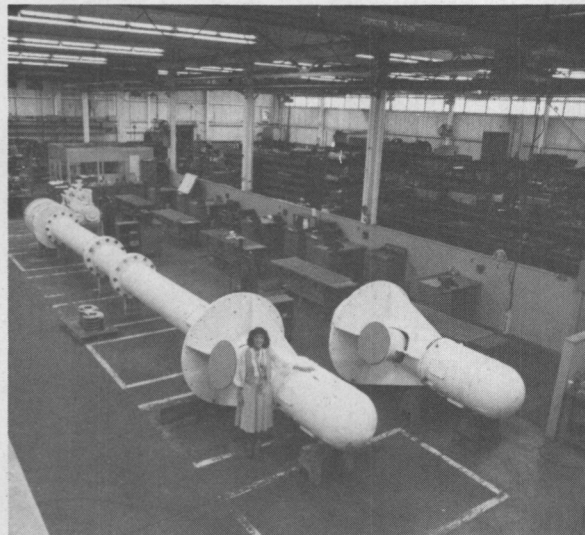
Fifty-foot Delaval GTS vertical pump system on the manufacturing floor at IMO Pump Division.
