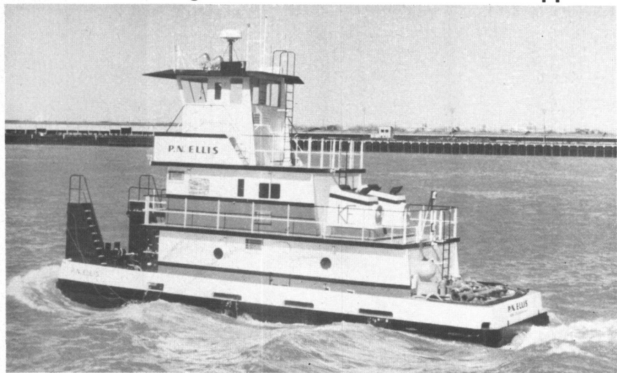
The 56-foot P.N. Ellis, powered by G.M. Detroit Diesel engines, has quarters for six men and complete live-aboard facilities.
