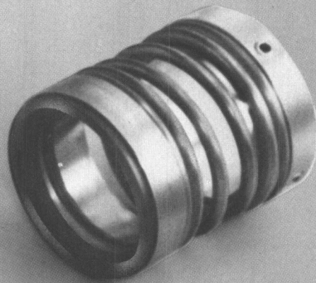
TYPE 670 — Good for broad range of applications aboard ship. This welded metal bellows seal will fit most existing cavities. All Hastelloy C construction for maximum corrosive resistance.
