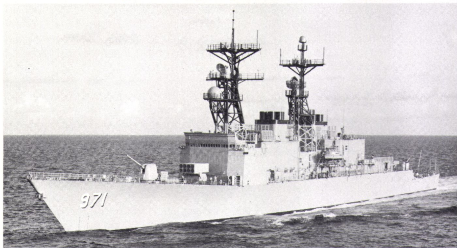
USS David R. Ray, DD-971, is powered by gas turbine engines and maintains speeds in excess of 30 knots.
