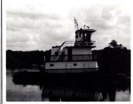
54'x20'x76", 2 years old, excellent condition, 800 horsepower, two Detroit Marine Diesel 12V-71 engines, 6:1 reduction, fully equipped including Konel Radar and 2 ship-to-shore radios. Contact Rogers Beall, P.O. Box 486, Slidell, Louisiana 70459. 504/641-2882
