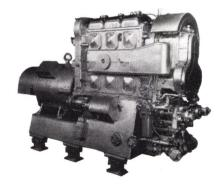
ENGINE: GM 3-268A-61/2×7-1200 RPM-80% power factor—electric starting. GENERATOR: 100 KW-440/ 3/60/1200 RPM — 161 amps. Dripproof — open — selfventilated. (Class "A' insulation stator — Class insulation on field). EXCITATION: 2 KW DC unit — 9' 1¾" long — 37" wide.
