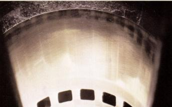
After 18,864 hours this cylinder liner from an EMD-12 645 E5 still shows original crosshatch marks. A tribute to the excellent wear
