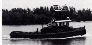
The Petchul-designed Hoosier State provides control both from the pilothouse and a fly-bridge station located on top of the pilothouse.
