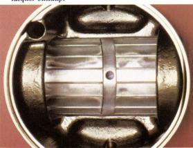
Much of the lead overlay is still intact on this wrist pin bushing from an EMD-12 645 E5 after 18,864 engine hours. No feathering of silver into the grooves. Tornus Oil has provided excellent lubrication.
