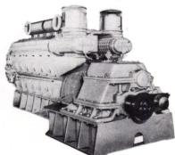
ENGINE: 12-567A — 8½x10 — VEE type — 2-cycle — 747 RPM—electric starting—serial Nos. 1041 & 1060. GEAR: Falk Air Flex—reverse and reduction—2.48:1 forward—2.52:1 reverse.
