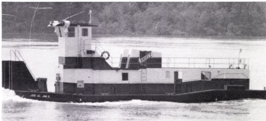
The Maxon-built M/V Joe Al Jim II is powered by Caterpillar diesels and equipped with a retractable pilothouse.
