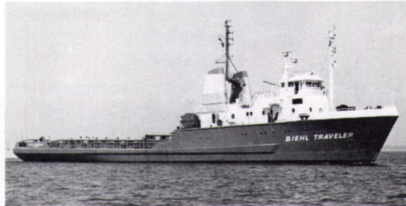
The Biehl Traveler is powered by two DeLaval Enterprise diesels, each producing 3,656 hp.
