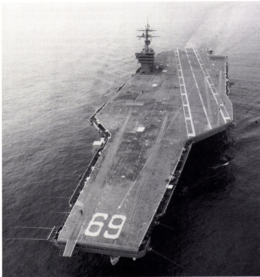
The Eisenhower's initial nuclear cores will provide enough fuel to carry out operations for the next 13 years.
