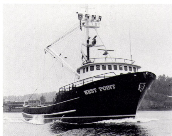
The 108-foot West Point powered by a Caterpillar diesel producing 850 bhp will operate in the Bering Sea.
