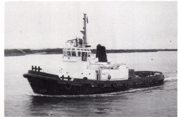
The M/T Broadsound, a 115-foot twin-screw tug powered by two 2,800-shp engines producing a bollard pull of 75 tons, is fitted with a high-pressure foam/water/jet spray fire monitor installed atop the wheelhouse. The tug was built for J. Fenwick & Co., Tugmasters of Sydney, Australia, for service in Hay Point, Queensland. Ten tugs have been built in all by Carrington Slipways for Fenwick. The M/T Broadsound was launched in December 1976.
