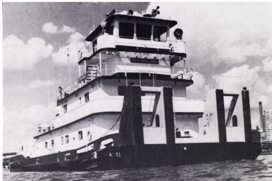
Representing a new class of Hillman-designed towboats, the twin-screw M/V Exxon Mobile is powered by Colt Industries, Fairbanks Morse diesels.
