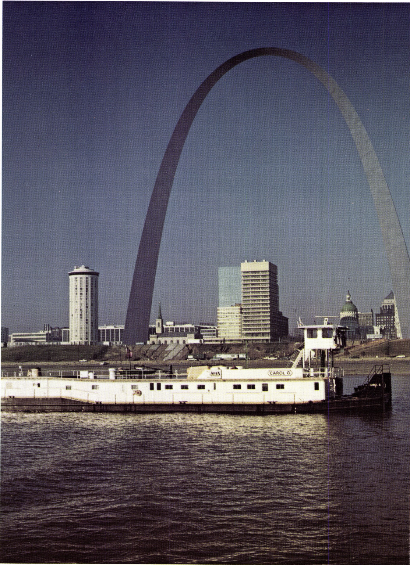
Carol G pushes her way up river easily. She is powered by two ALCO 251 diesels, each rated at 2200 BHP. The CAROL G is Apex Barge Company's newest vessel.
