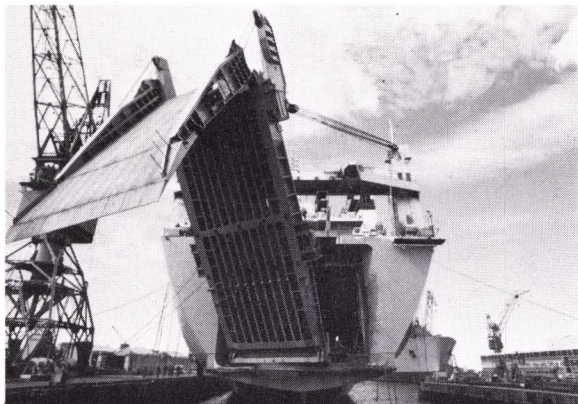
The MacGregor slewing ramp was recently tested in Kiel. It is shown here being slewed to port.
