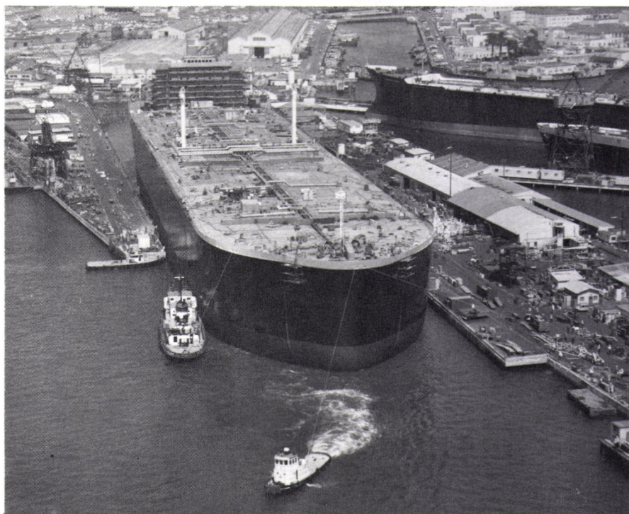
Hull 405, 188,500-deadweight-ton San Diego-Class tanker, is hauled from the graving dock of National Steel and Shipbuilding (NASSCO) of San Diego, Calif. The new tanker is the first of four to be designed and built by NASSCO. Hull 405 and 406 are for long-term use by Shell Oil Company. Hull 408 and 409 will be built for Atlantic Richfield Company. All of the tankers will be used in the Alaskan oil trade.
