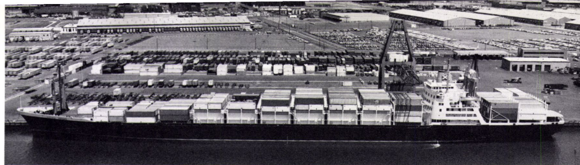
SS Austral Entente at Port Newark after jumboizing
