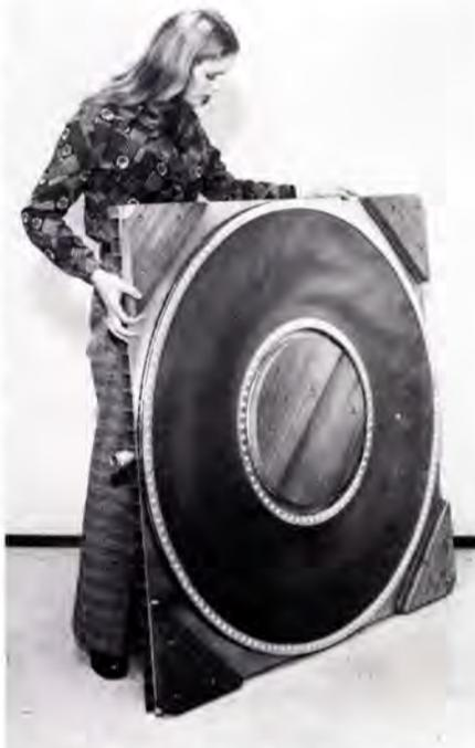
Aero-Caster waterfilm load module used by Vancouver Shipyards is 4 feet square, 3 inches thick, and weighs 170 pounds.
