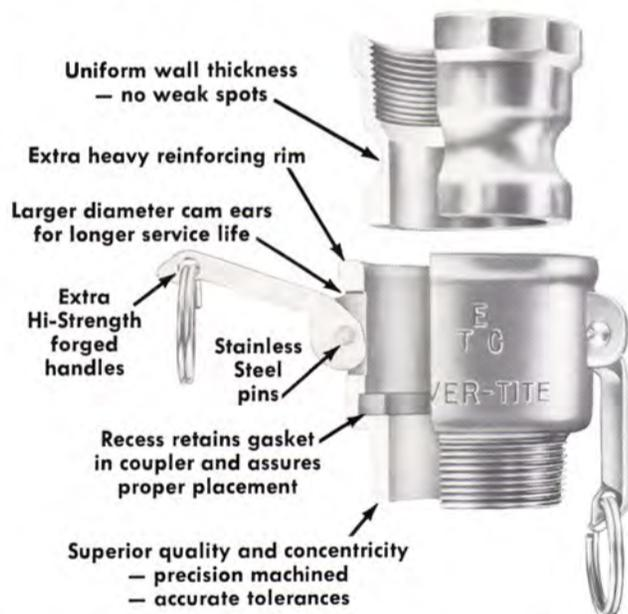
Sizes from 1/2" to 10". Choice of metals, gaskets, male or female NPT or straight threads, hose shanks, flanges, or machined for socket or butt weld. Also valved couplings to connect or disconnect full lines without spillage.
