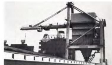
**Bulk Unloaders**—One of the world's largest Alumina unloaders, designed by PACECO with dust enclosure over hopper and sealed clamshell bucket. Handles 1000 Long Tons per hour with minimum loss of material.
