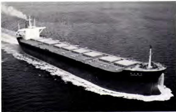
The 136,000-dwt Amagisan Maru is shown above while on trials. The Kawasaki-built ore carrier recorded 17.97 knots on trials. It is fitted with a nozzle propeller.
