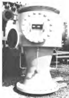
An 18" PrimaVac Unit for the 12,000 gpm cargo pumps on the 86,000 dwt tankers.
