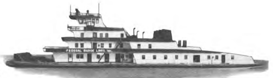
Keene Marine Discharge Control Systems are installed on Federal Barge Line's two largest vessels, the 4-engine, 9000-hp, 184-foot M.V. America and its sister ship M.V. United States (shown here).
