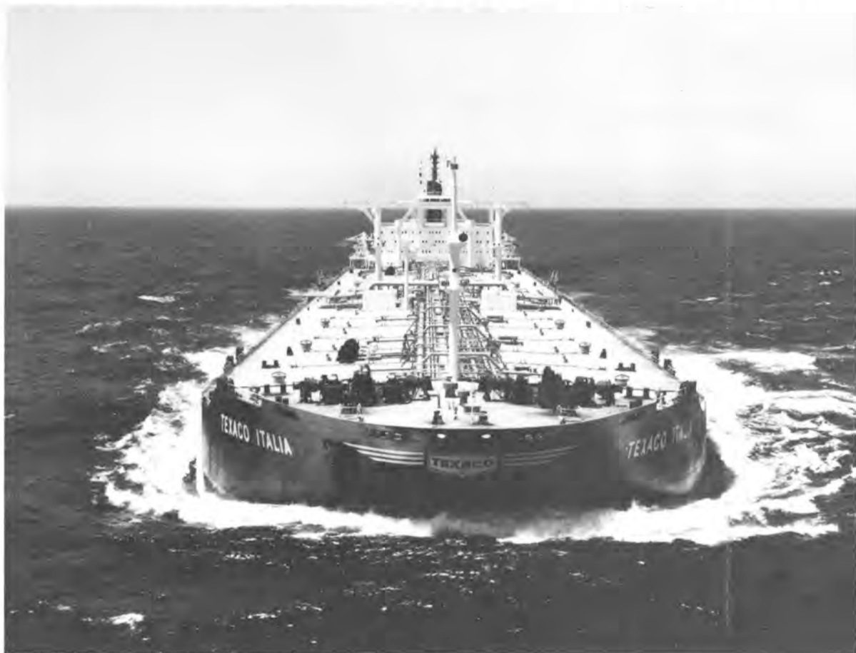
The Texaco Italia, shown during her sea trials, has a cargo capacity of 2,000,000 barrels of crude oil on a single voyage, with a service speed of about 15.8 knots.
