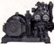
Two stage—water cooled—single acting verticle type—10 CFM—600 lbs. Type 30—Class T. Ingersoll-Rand Compressor—4x1½ x3½ @ 630 RPM. Motor 7½ HP—440/3/60—1750 RPM—complete with starter—intercoolers and aftercoolers.
