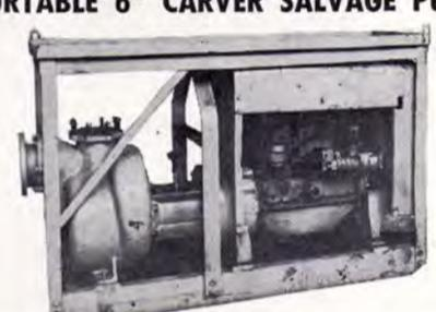
Reconditioned—mounted in portable steel frame. 1750 RPM—1100 GPM @ 100' head; 1500 GPM @ 70' head; 1800 GPM @ 50' head; 2100 GPM @ 20' head. Leroi gas engine—model D-201P3 —4 x 4—1750 RPM—hand crank—wt. 600 lbs.
