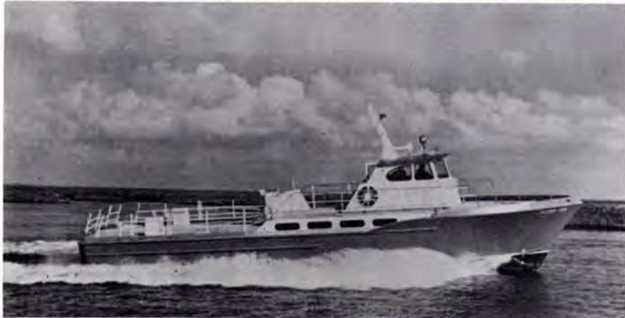
**ON THE COVER:** The Gacship IV is powered by three Caterpillar D-343 turbocharged after-cooled engines and can reach a speed of 23 mph.
