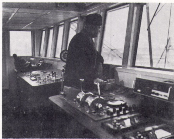
Capt. Bill E. Jeffery shown at the wheelhouse controls during trials. He can control the propeller rpm and engine speed, plus the bow thrusters from the pilot house.
