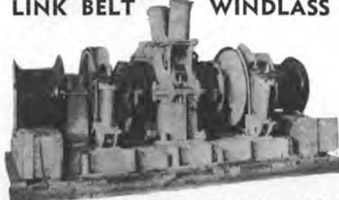
Below deck motor drive. Double wildcat—driven by 50 HP 230 VDC motor with vertical shaft and worm drive. Single speed—handles 7000 lb anchors and 60 fathoms of 1½" chain at 7 fathoms per minute. Wildcat centers 56". Complete with all controls and warping features. Total weight 27,500 lbs. With spares.
