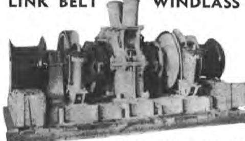
Below deck motor drive. Double wildcat—driven by 50 HP 230 VDC motor with vertical shaft and worm drive. Single speed—handles 7000 lb anchors and 60 fathoms of 1 5/8" chain at 7 fathoms per minute. Wildcat centers 56". Complete with all controls and warping features. Total weight 27,500 lbs. With spares.
