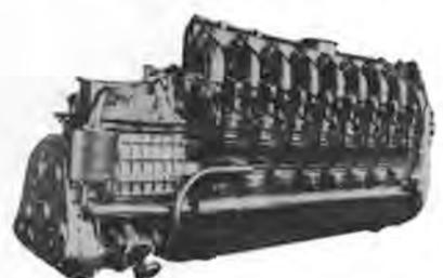
Complete, clean and in very good condition. As removed from U.S. Naval vessels. 1700 HP @ 750 R.P.M. Your inspection invited.
