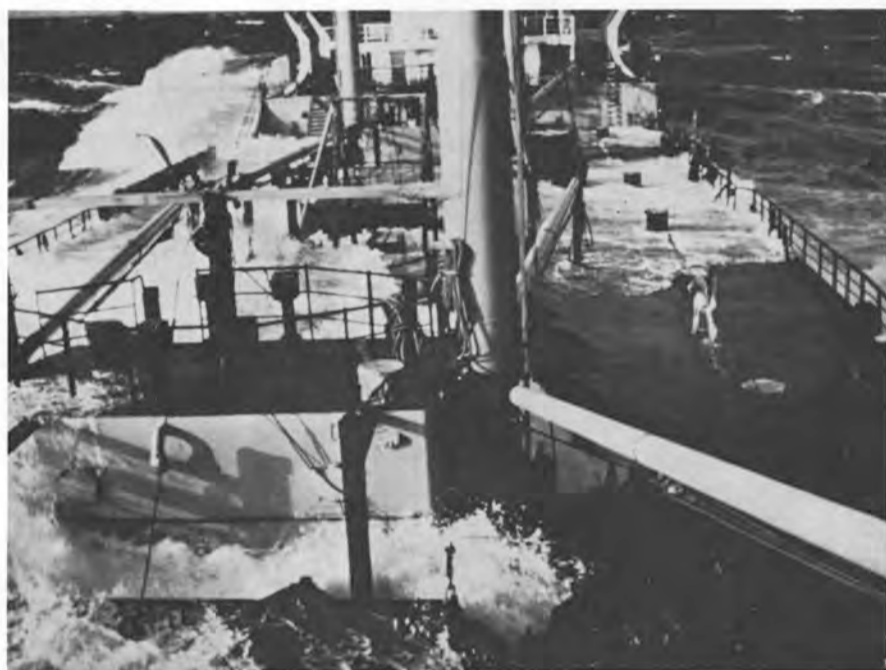
Green seas over the bow provided a severe, prolonged test, particularly on the #1 hatch.
