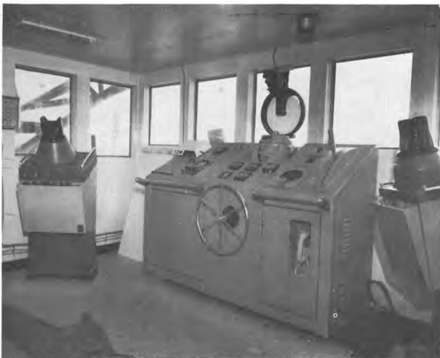
Radar scanners flank the bridge console in the pilothouse. Course keeping is maintained through a rate control gyro and gyropilot, and steering is by fine differential RPM control. No rudders are fitted to the rig as the control of the speed and direction of rotation of the propellers provide excellent control under power.
