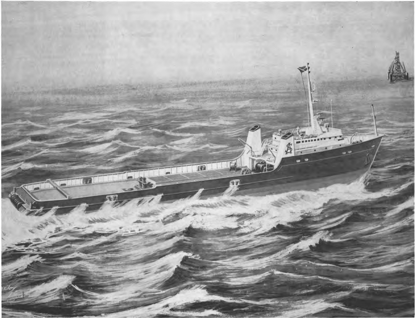
Artist's conception of tug/supply vessels being built by Todd for Allseas of Panama, Inc. The craft will be 228 feet overall.
