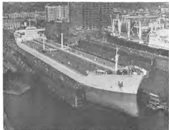
The Asopos was docked stern first, with the bow overhanging the river by 114 feet.
