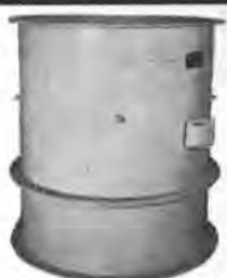
Made by Joy Manufacturing Co.—A30A4W6. MOTOR: 25/14 HP—440/3/60—36-20.4 amps—1200/1900 RPM.
