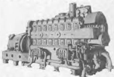
ENGINE: 8-268A—6 1/2" bore x 7" stroke—1200 RPM—driving 200 KW Westinghouse generator—440 volts—3-phase—60 cycle—321 amps—80% power factor at 1200 RPM.
