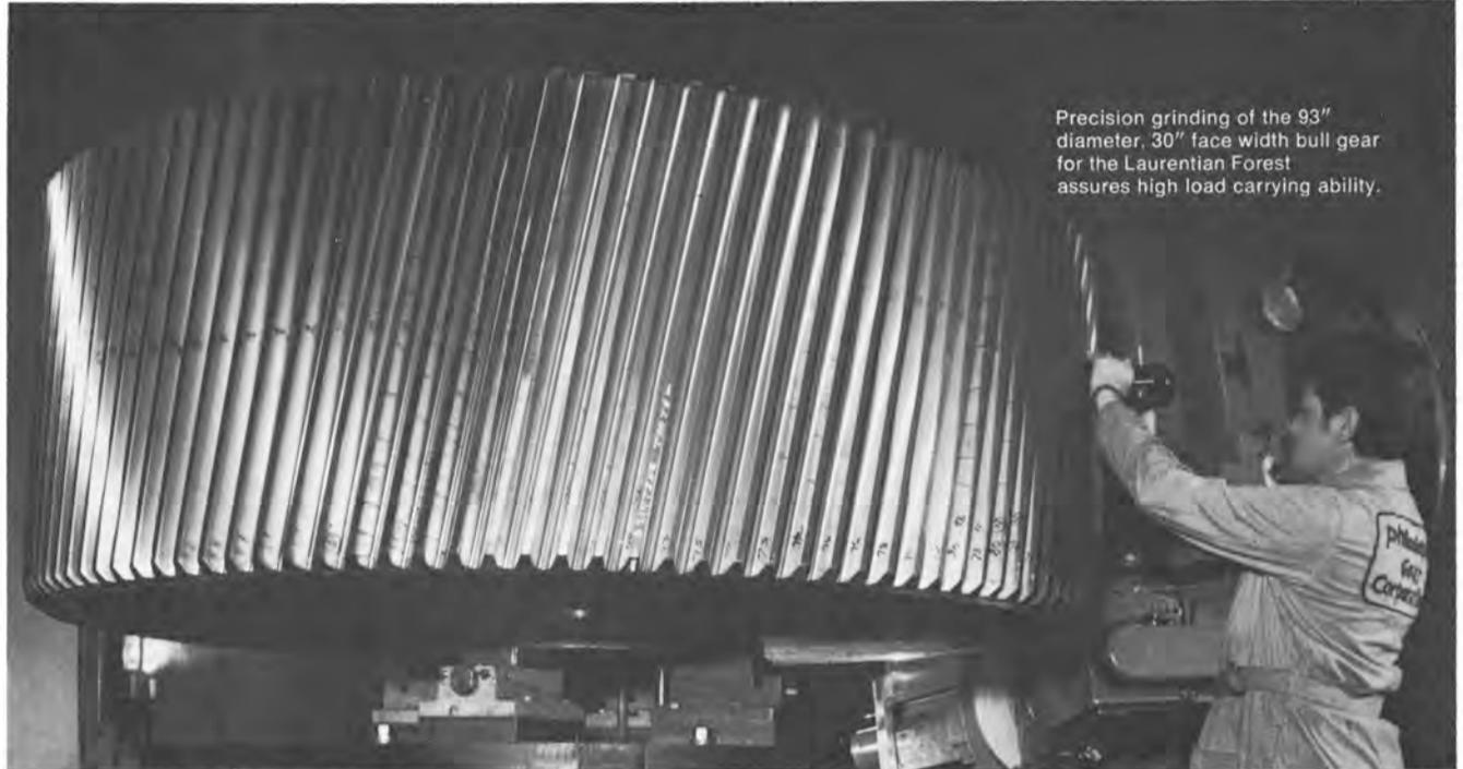
Precision grinding of the 93" diameter, 30" face width bull gear for the Laurentian Forest assures high load carrying ability.
