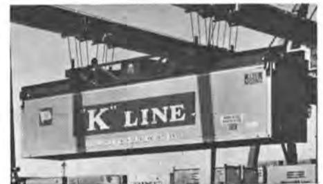
Universal expandable spreader — for gantry crane (above) or side-loading truck (below).
