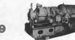
LOW-PRESSURE UNUSED 300 KW G.E. 120/240 VOLT DC TURBO-GENERATOR SET
