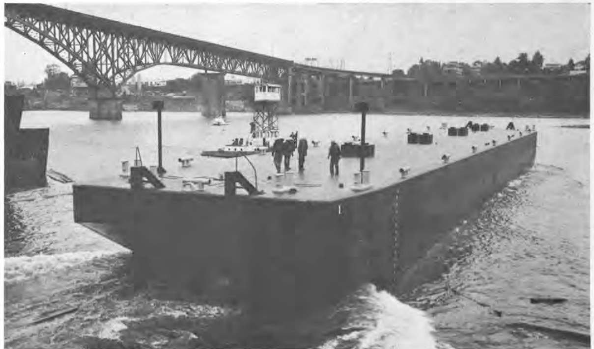
ZIDELL'S 140TH BARGE: Zidell Explorations, Inc., Portland, Ore., has launched its 140th barge since going into production in 1961. The latest is Tidewater Barge 1, shown above, built for Tidewater Barge Lines, largest barge operator on the Upper Columbia River. Tidewater 1 measures 242 feet by 42 feet by 16 feet 6 inches, and is designed to haul up to 25,000 barrels of petroleum from Portland to the Upper Columbia. Separate piping and pumping for each cargo compartment will permit carrying as many as eight different petroleum products simultaneously, with no problem of contamination in loading or unloading. According to a Tidewater spokesman, who placed the cost of the barge at $500,000, this is a unique feature on the Columbia. Tidewater 1 is the ninth barge built by Zidell for Tidewater since 1970. The previous eight were all grain barges. In addition to its Upper Columbia operations, Tidewater also operates between the Columbia and California. Its headquarters are at Vancouver, Wash. Barges previously constructed by Zidell at its Portland yard have ranged from a 122-foot deck cargo barge to a 300-foot derrick barge packing a deck crane with a 500-ton lift capacity and certified for unlimited ocean service.
