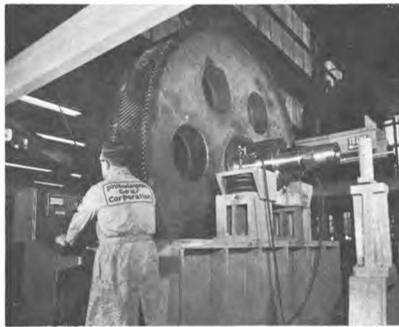
Dynamic balancing one of the three 20-ton bull gears for the icebreaker drives. Each gear was 135 inches in diameter and was tested to specification Mil-Std-167.
