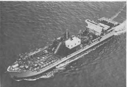
The Petrobras II leaves the Tamano yard of Mitsui upon acceptance of her owners. The self-propelled drilling rig is designed to rotate its amidships drilling rig.
