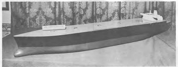
The LNGs to be built by Avondale will have a single flush deck on which the cargo-handling system is arranged, providing optimum visibility from the bridge.
