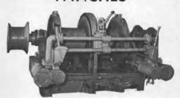
Drum 8500 lbs @ not less than 120 FPM; 13,000 lbs at no specific speed. Gypsy head 22,500 lbs static pull. Foot brake to hold 17,000 lb. pull. Steam cylinders with standard 250 PSI.
