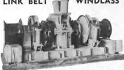
Below deck motor drive. Double wildcat—driven by 50 HP 230 VDC motor with vertical shoft and worm drive. Single speed—handles 7000 lb anchors and 60 fathoms of 13/6" chain at 7 fathoms per minute. Wildcat centers 56". Complete with all controls and warping features. Total weight 27,500 lbs. With spares.
