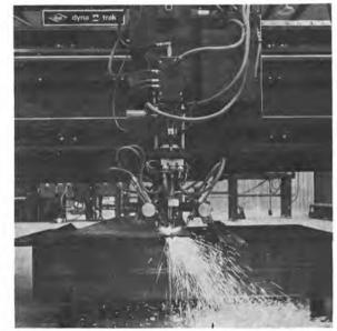
Each work station has a torch mounted vertical to the work piece and bevel torches oriented at angles to the work surface.
