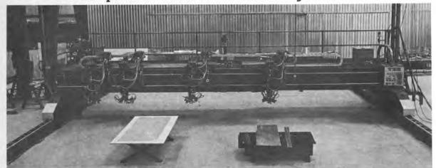
Overall view of Heath/Liquid flame cutting machine built for Sun Shipbuilding & Dry Dock Co. The machine has four three-torch cutting stations, and it can simultaneously perform edge profile work on two 16-foot-wide plates.
