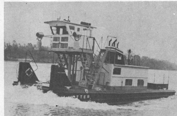
The elevating pilothouse on the Otter affords the operator an eye level exceeding 28 feet at peak height.
