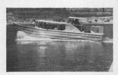
It's easy to see why JacuzziJet propulsion significantly reduces operation costs. With no protruding parts beneath the hull, the chances of incurring expensive damage are greatly reduced.
