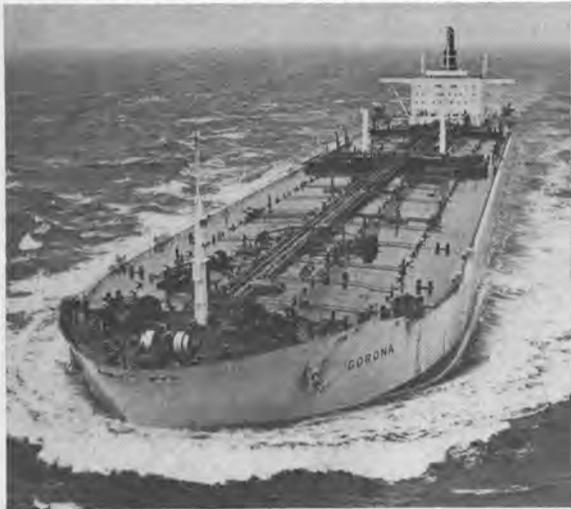
The Gotaverken-built T/T Corona has been built to the highest class of Det norske Veritas and classed EO (unmanned engine room).
