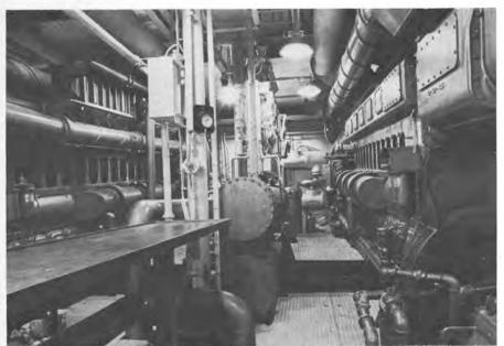
Looking forward in the engine room between the two Fairbanks-Morse diesel engines indicates ample work areas. These engines are remotely controlled from the bridge.
