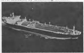
The Gadinia, 75,000-cubic-meter capacity, is the first in a series of five LNG tankers of the same design. All five vessels will be used to transport LNG from Brunei to Japan.
