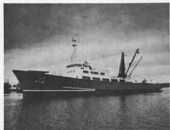
"MARGARET L"—The world's largest and most beautiful Tuna Seiner: Length: 262', Beam: 45'. Capacity: 2000 ton. Horsepower: 720 SHP. Range: 4000 miles.
