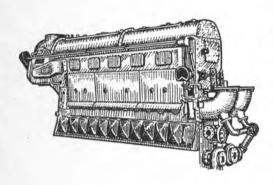
MATCHED PAIR . . . FAIRBANKS MORSE MODEL 38D8-1/8—1 Port; 1 Starboard. Used condition, 1800 HP, 800 RPM, 2 cycle, 8½" bore, 10" stroke, Air Start. Complete with Westinghouse Reduction Gears, 2.216:1 ratio—with Hydraulic Coupling.
