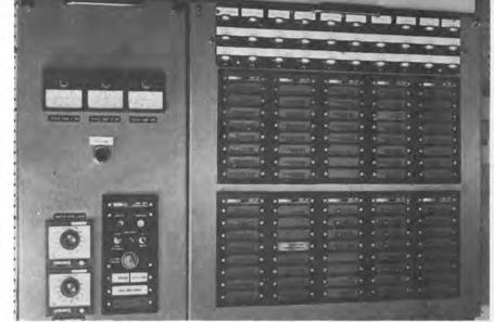
The ITT Decca Marine monitoring panel covers 76 points throughout the vessel. This system assures efficient and trouble-free operation during critical fishing.
