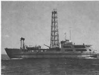
"ALCOA SEAPROBE"—The world's largest all-aluminum Oceanograph Research Vessel: Length: 243', Beam: 50', Derrick: 132' above W.L., Propulsion: Two cycloidal omni-directional propulsion units, Range: 6600 miles.
