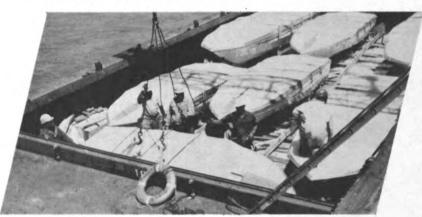
Seven 17 to 22-foot-long inboard/outboard boats are stowed over flour, carborundum, resin, machinery parts and other general cargo.
