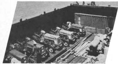
Standard container occupies portion of LASH barge loaded with farm vehicles, steel rods and miscellaneous general cargo.
