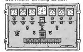
Kockums Burner Control (KBC): an automatic, all-electronic burner management system for safe, simple boiler/burner light up and shut down. Every start and stop sequence is automatic, activated by a single button. The light-up sequence can be varied as required.
