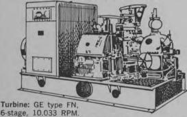
Reduction gear: GE triple-helix, triple reduction, 10033/1200 RPM. Generator: GE type ATI, 600 KW, 6-pole, 0.8 pf, 450 VAC, 3 phase, 60 cycle, 1200 RPM. Exciter: GE type MPLI, 7.5 KW, 120 VDC, direct connected. Air cooler: Surface type, for generator, complete with control panel.
