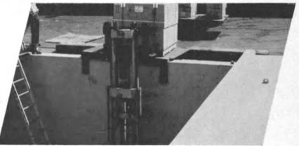
Fork lift-to-fork lift transfer of packaged cargo is another advantage of LASH cargo handling.
