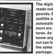
The digital indicator reads out directly in pounds. Both visual and audible alarms and an automatic tare adjustment are standard features. As an option, a boom angle digital readout can be included in the same indicator
