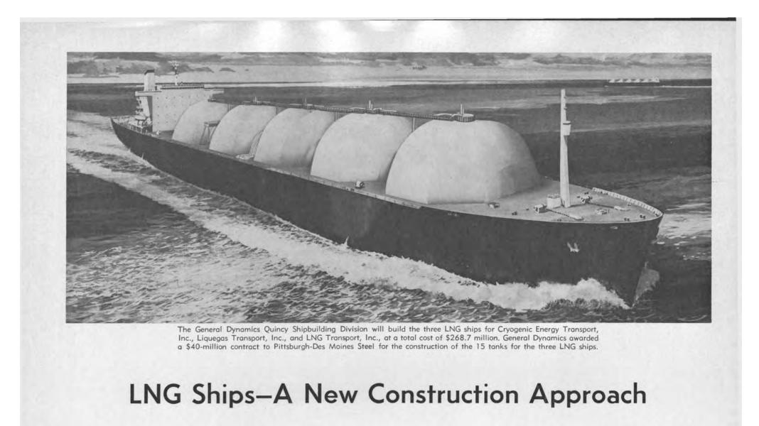
U.S. Shipyard And Cryogenic Tank Builder Team Up To Offer An Improved Method Of LNG Ship Construction
