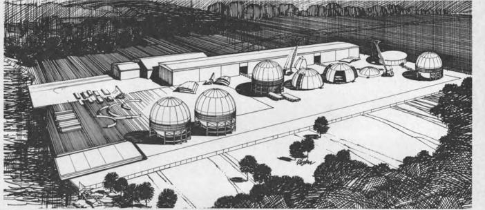
Figure 2-The proposed manufacturing plant with separate areas for the forming and trimming of plates, subassembly of sphere sections and final assembly. At the plant, the spheres will be loaded onto the barges without the use of lifting equipment.
