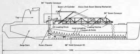
Schematic drawing of tug-barge cargo transporter shows layout of materials handling system which includes a total of 198 unloading hoppers, dual 66-inch-wide hold conveyors, unique rotary elevator, transfer conveyor and 250-foot boom conveyor.
