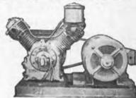
2—GARDNER-DENVER, 150 CFM, 125 PSI, Class WB, Size 7x5 3/4 x5, with Diehl Motors, 45 HP, 230 Volts DC, 870 RPM, 167 Amperes.
