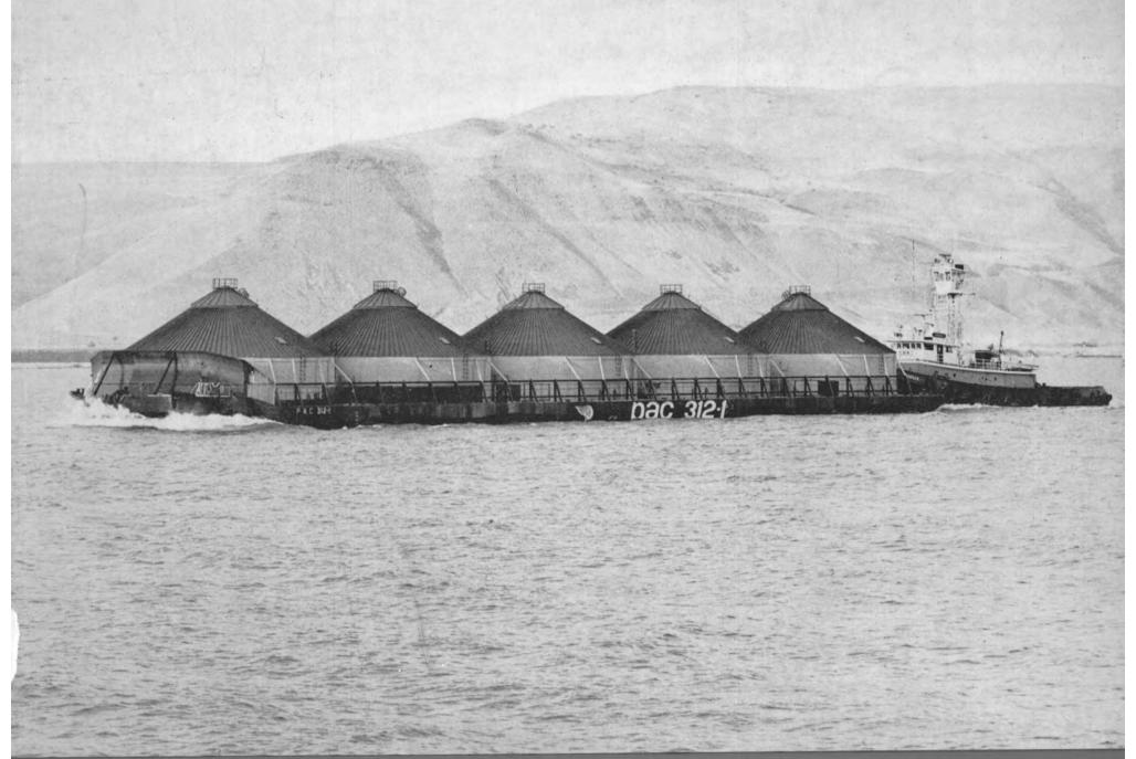
**Grain In Five Deck-Mounted Tanks** Transported In Oceangoing Service Using One PAC Barge And Tug (SEE PAGE 6)
