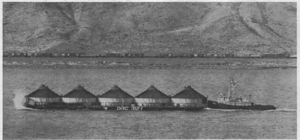
The PAC tug Sioux pushed the huge barge 388 miles from Central Ferry, Wash., to Astoria, Ore. and then switched to hawser towing for the trip southward in the Pacific. Some trips will also be made to Hawaii under the charter.
