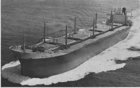
The Panmax-type 60,503-dwt general-bulk carrier Evelyn is shown undergoing sea trials. The Evelyn is the fourth in a series of 13 similar ships being built by Hitachi-Zosen.
