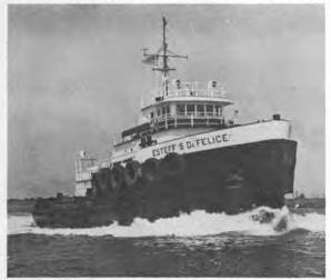
The new tug, designed primarily for work with the offshore industry, has a fuel oil capacity of 170,000 gallons for long-range and extended operations.
