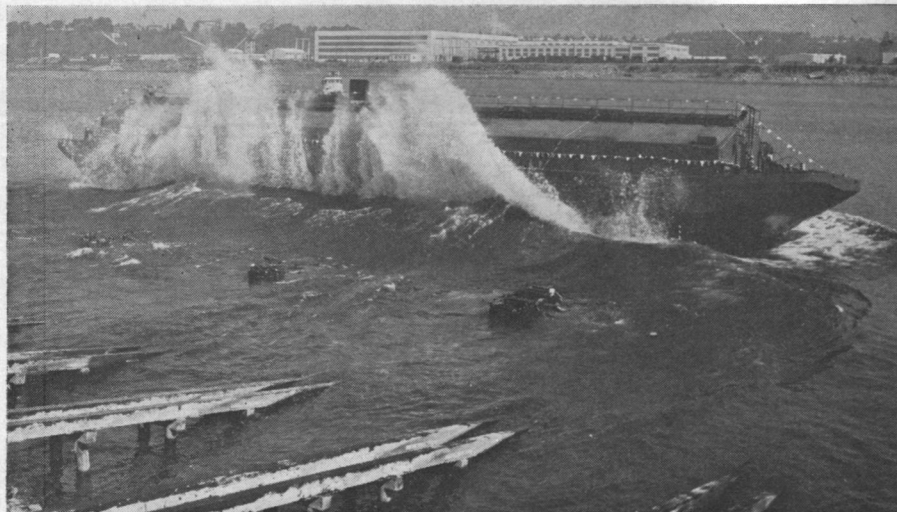
SHAYER GRAIN BARGE: The second of two grain barges built this year for Shaver Transportation Company of Portland, Ore., is shown being side-launched recently at the yard of the builder, Gunderson, Inc., Portland-based marine construction firm. Sponsored by Mrs. Luella Shaver, wife of George Shaver, the barge, named ST-36, measures 207 feet by 42 feet by 15 feet and will be used on the upper Columbia and Willamette Rivers, primarily by Western Grain Exchange, Inc. The barge has a grain capacity of 2,700 tons of wheat or 2,200 tons of barley. According to Mr. Shaver, executive vice president of the West Coast transportation firm, the ST-36 was built according to American Bureau of Shipping regulations, insuring high quality design and construction. Portland naval architects Don Hudson & Associates were the design agents. Doug Hendrix of the Portland office of the American Bureau of Shipping was the principal surveyor. Gunderson, Inc., is a subsidiary of the FMC Corporation, San Jose, Calif.
