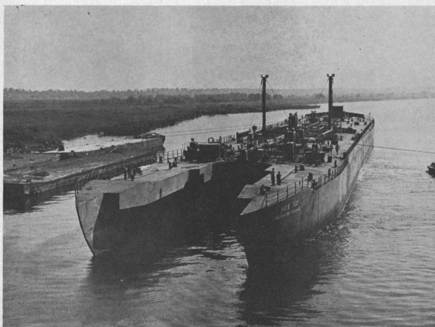
The I.O.S. 3301, built by Alabama Dry Dock and Shipbuilding, measures 532 feet in length, has a beam of 87 feet, and an unusually deep stern slot for the powerful tug.
