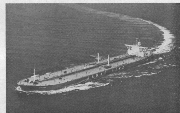
HITACHI TANKER DELIVERY: The 232,079-dwt oil tanker Sanko Lake, constructed at Hitachi Zosen's Sakai Shipyard was recently delivered to Regent Shipping Inc., Liberia. Classed by Bureau Veritas, the approximate measurements of the tanker are: length, 1,000 feet; breadth, 167 feet, and depth, 85 feet. The vessel is powered by a Hitachi Zosen UA-360 type marine steam turbine with a maximum output of 36,000-horsepower providing a trial speed of 16.63 knots.
