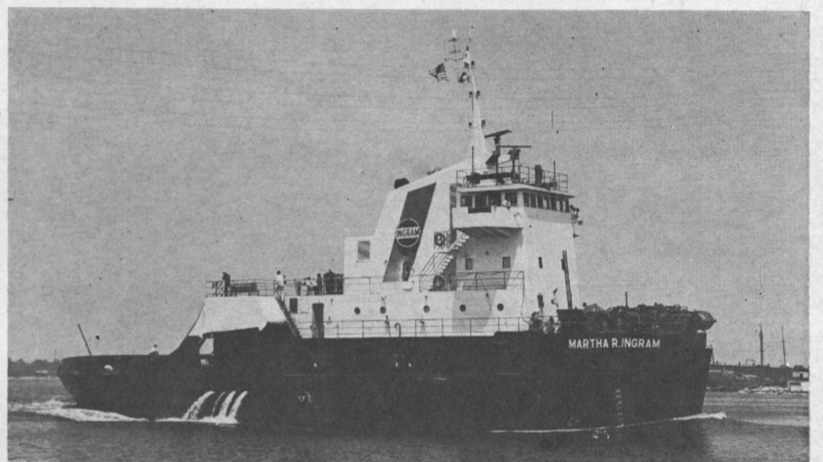
The 11,250-hp Martha R. Ingram, built by Southern Shipbuilding, Slidell, La., is capable of pushing the 285,500-barrel barge at a speed of 14 knots at full load draft.
