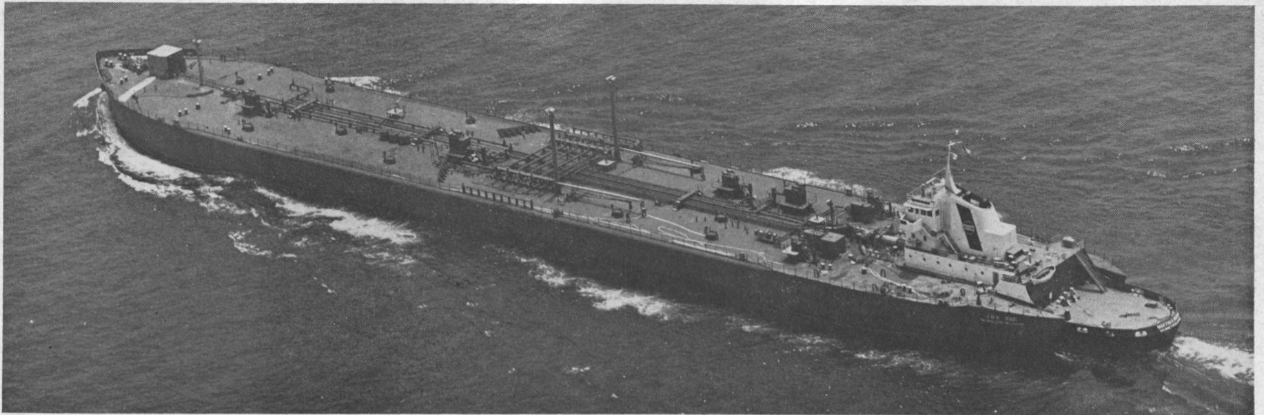
The completely integrated tug-barge unit, with a length of 620 feet 6 inches and a deadweight of 36,530 tons, resembles a self-propelled tanker.
