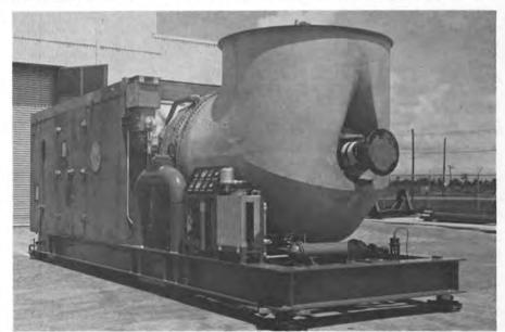
One of the Euroliner's powerplants ready for shipment. The complete unit is mounted on its frame for easy handling. This unit was shipped in a standard 40-foot container.
