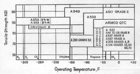
Figure 1—Relative qualities of steels for use in liquefied gas product service.
