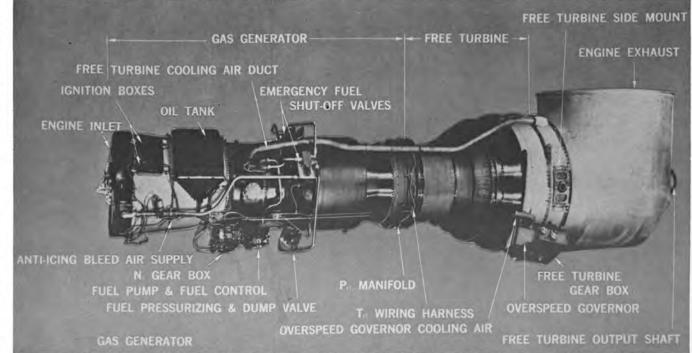
Annotated view of the FT4 marine gas turbine with the gas generator on the left and the free turbine on the right.
