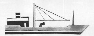
Our new barge, the MV Taboga, is the largest in the Panama Canal area. It has a 6,500 ton, 46,000 barrel capacity. (Over double any of our other barges.) And an increased pumping rate of 1,000 tons per hour.
