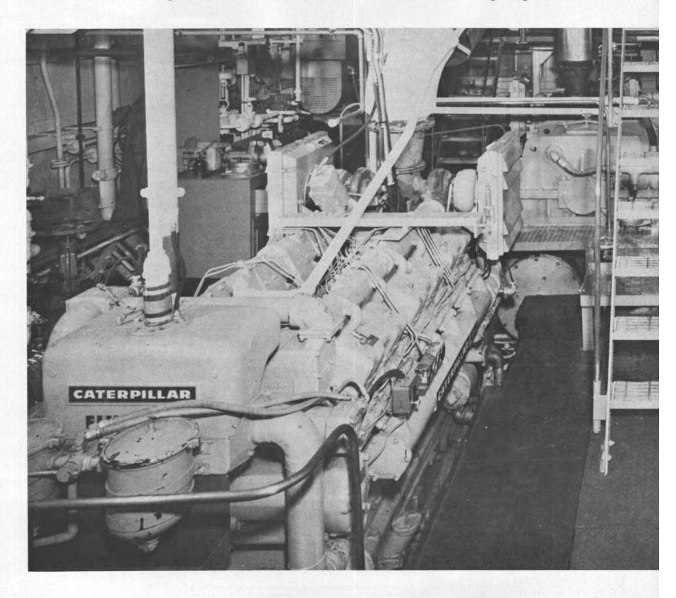
Engine drives the towing winch through a torque converter. Ask your Cat Dealer to help plan a Cat Diesel compound installation for you. He has all you need: Diesels 85 to 1425 hp. Marine gears. Electric Sets 40 to 900 kw. All Caterpillar-built, with dealer service available the world over.
