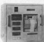
The Bell Logger records automatically whenever a control is moved. Precise digital printout of Throttle Control, Engine Order, Reply, actual Shaft RPM, or other data is presented digitally and permanently recorded with the exact time. It can also double as the Ship's Master Clock.
