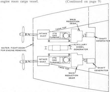
Simplified arrangement plan of the Euroliner's engine room shows the main units.
