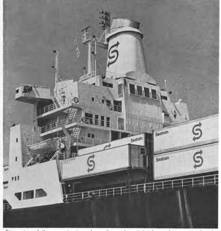
Stern view of the superstructure shows the engine air-intake enclosures on aft side.
