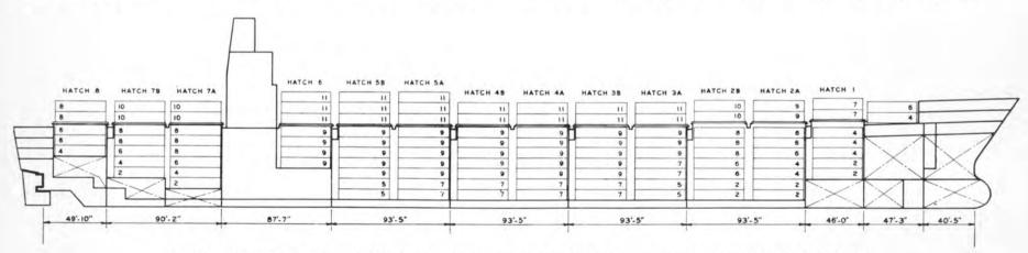
Inboard profile of the Euroliner indicates the container-stowage arrangement and the small volume needed for the engine room.
