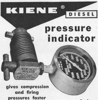
The Model K-100 Kiene Pressure Indicator accurately measures compression and firing pressures — assures proper maintenance of diesel engines — helps prevent costly down time. Only one moving part—no friction or inertia effects—no complicated adjustments. Steel carrying case and service tools included.
