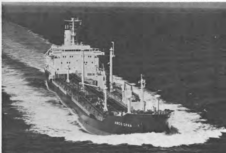
The Anco Span, one of five sisterships built by Eriksberg Mek. Verkstad for Anco Tanker Service, is a 23,500-dwt parcel tanker. It has a length overall of 556 feet 6 inches, a beam of 81 feet 3 inches and a depth of 41 feet. The total capacity of the cargo tanks is 191,238 barrels. Propulsion is by a seven-cylinder, single-acting, turbo-charged diesel of the Eriksberg's Burmeister and Wain type, developing 11,500 bhp.
