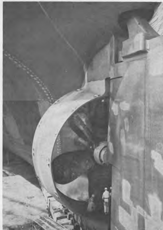
View of world's largest nozzle propeller installed on large tanker by Kawasaki Heavy Industries' Sakaide yard.
