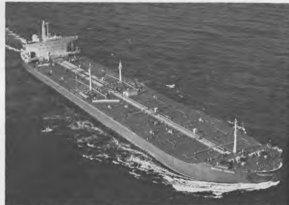
The 215,782-dwt tanker Golar Nichu, shown on trials off Japan, attained an average sea speed of 16.61 knots.
