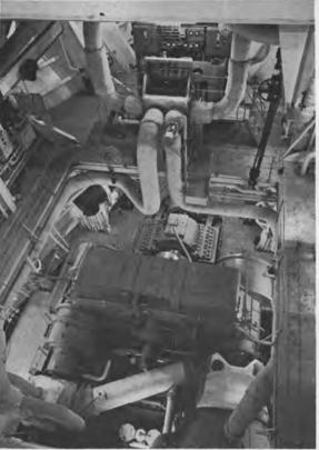
Overall engine room view looking aft towards the maneuvering valves shows reduction gears and thrust bearing.
