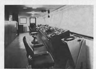
The large wheelhouse has navlgating, steering and machinery controls in one console along forward bulkhead.
