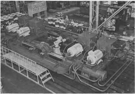
World's largest electro-hydraulic steering gear assembled in Kawasaki Heavy Industries' shop for testing. The overall width of the unit is 33 feet 11 inches and it measures 17 feet 4 inches in the fore-and-aft direction. Its height is 6 feet 5 inches.
