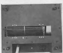
View of programmable control unit, showing some of the 40 punched metallized cards pre-programmed for particular frequencies. Cards can be changed in minutes, even at sea.
