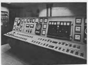
The engine room main control console is located in the machinery control room on the intermediate platform.
