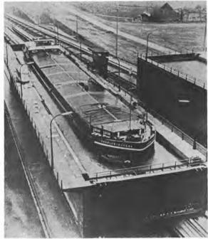
A barge in a portable tank is being transported overland in Belgium. A similar method is proposed to complete the Cross-Florida Barge Canal utilizing the Syncrolift System.
