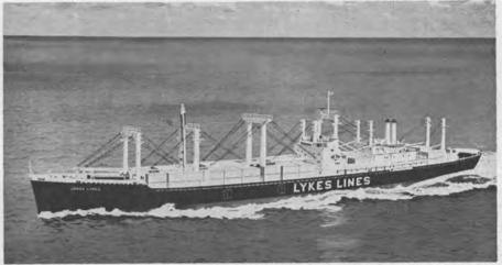
This is how the newly lengthened ships of the fleet of Lykes Bros. Steamship Co., Inc., look after adding a new 97-foot mid-body section. Todd Shipyards in Galveston are converting the ships at a cost of \$30 million.
