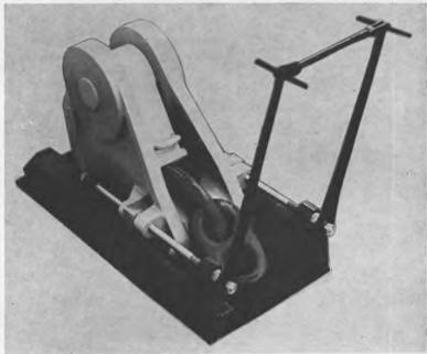
One unit can eliminate devil's claws, turnbuckles, bow stoppers and, it utilizes less space. The one stopper that serves the dual purpose of transferring chain load to the vessel's structure and houses the chain in a snugly stowed position.
