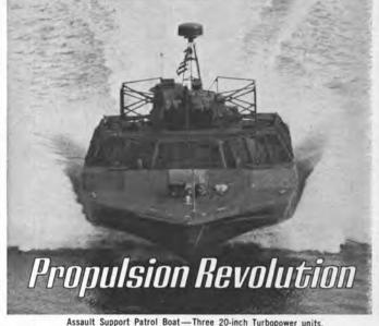
Assault Support Patrol Boat-Three 20-inch Turbopower units
